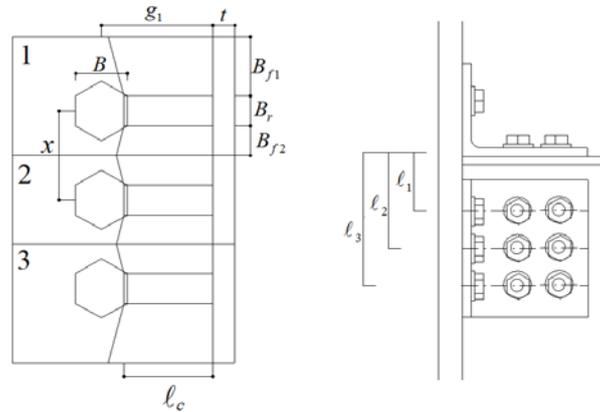
Figure 11. Segmental beam model for web angle
