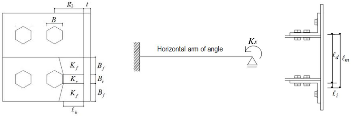
**Figure 7.** Segmental beam model for horizontal arm of top angle
