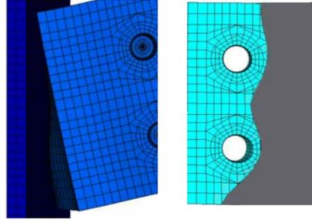
**Figure 10.** Separation characteristic in the web
