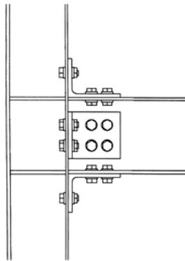
Figure 4. Semi-rigid connection
