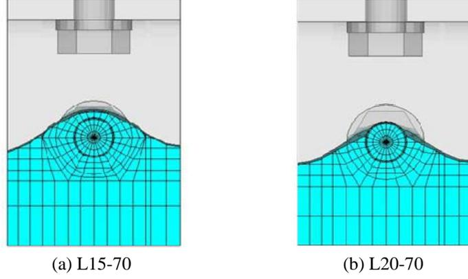
**Figure 6.** Separation pattern in the vicinity of bolt area
