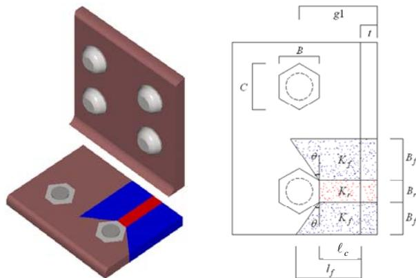
Figure 5. Segmental beam model for vertical arm of top angle
