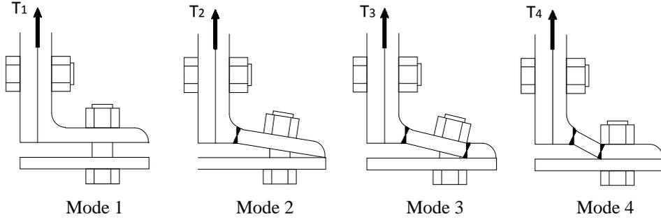
**Figure 8.** Failure modes for semi-rigid connection
