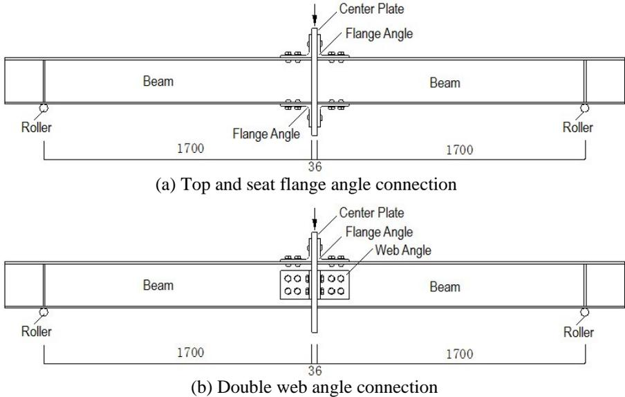
**Figure 1.** Bending test specimens
