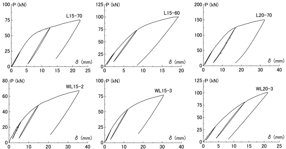
**Figure 3.** Load versus displacement curves for bending tests**Table 2.2.** Results of bending tests
