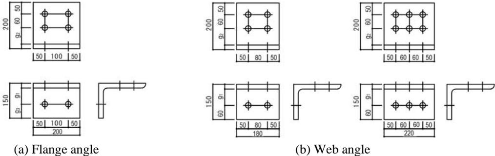
**Figure 2.** Connection details for specimen of both types
