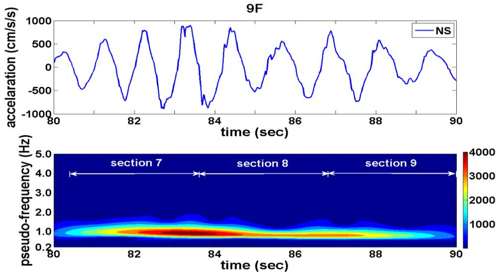
(a) Acceleration waveform at 9F and wavelet transform
