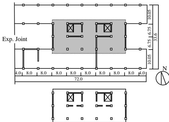
Figure 2. Plans at the 1<sup>st</sup> floor (top) and the 3<sup>rd</sup> floor (bottom)
