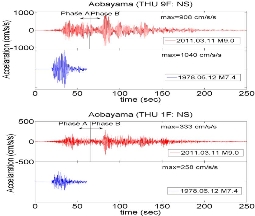
Figure 6. Comparison of observed records of 2011 Tohoku earthquake and 1978 Miyagi-ken Oki earthquake (NS direction)
