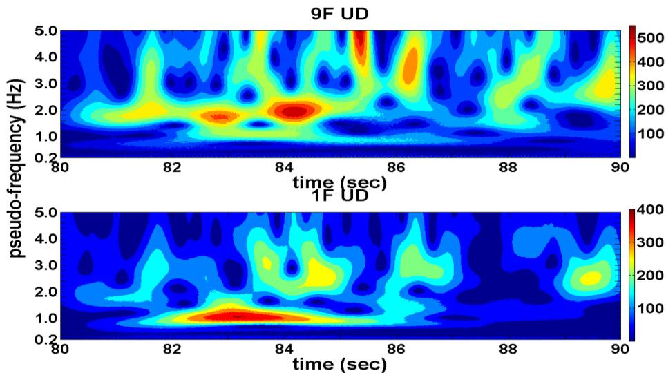
(b) Wavelet transforms of acceleration in the vertical direction at 9F and 1F.
