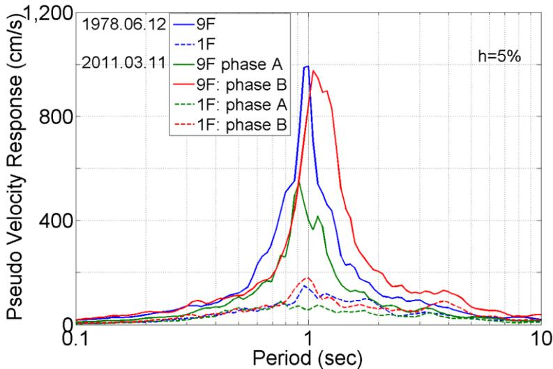
Figure 7. Comparison of response spectra of 2011 Tohoku earthquake and 1978 Miyagi-ken Oki earthquake
