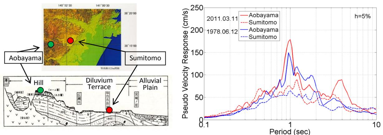
Figure1. Geological information and site specific spectral amplification in Aobayama hill, Sendai
