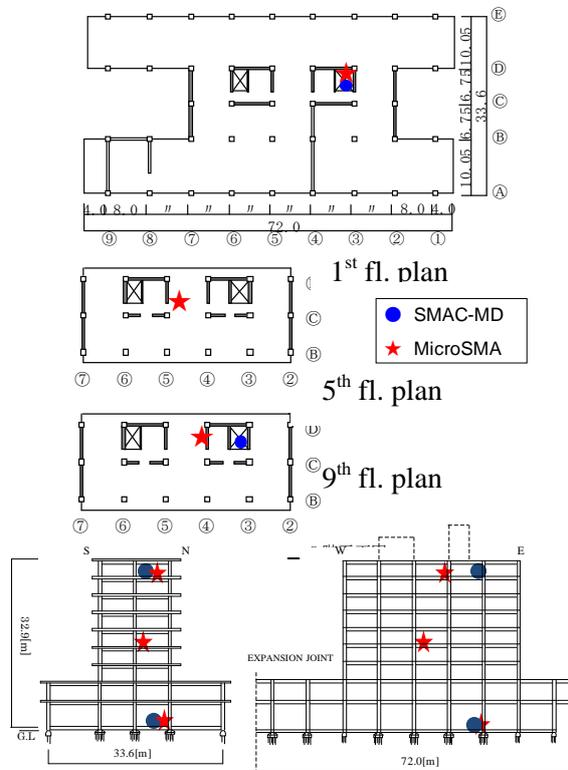
Figure 4. Configuration of THU Building and Sensor location
