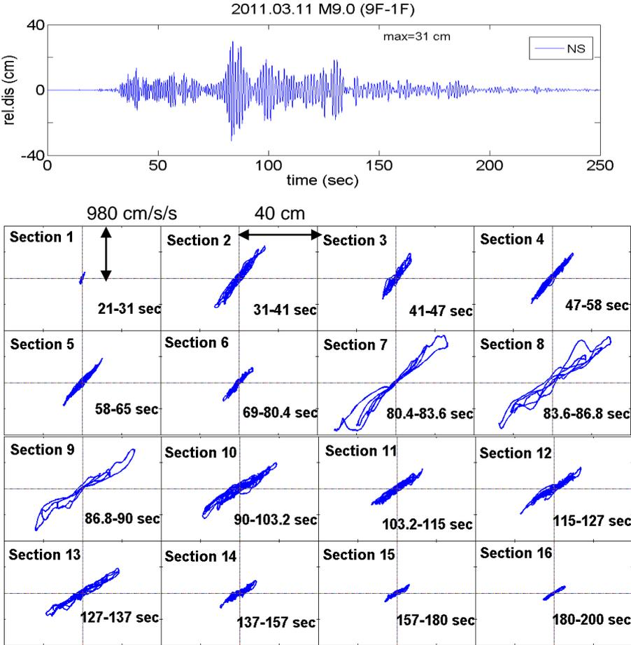
Figure 8. Relative displacement waveform and hysteresis loops for each time section (NS-Direction)
