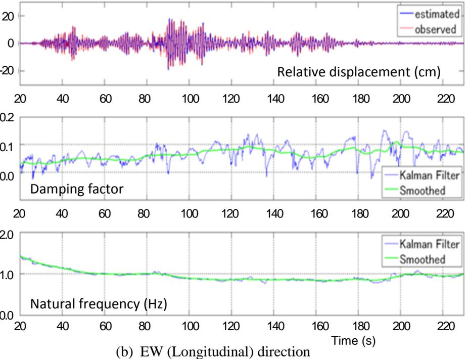
Figure 10. Identified damping and natural frequency in the horizontal two directions
