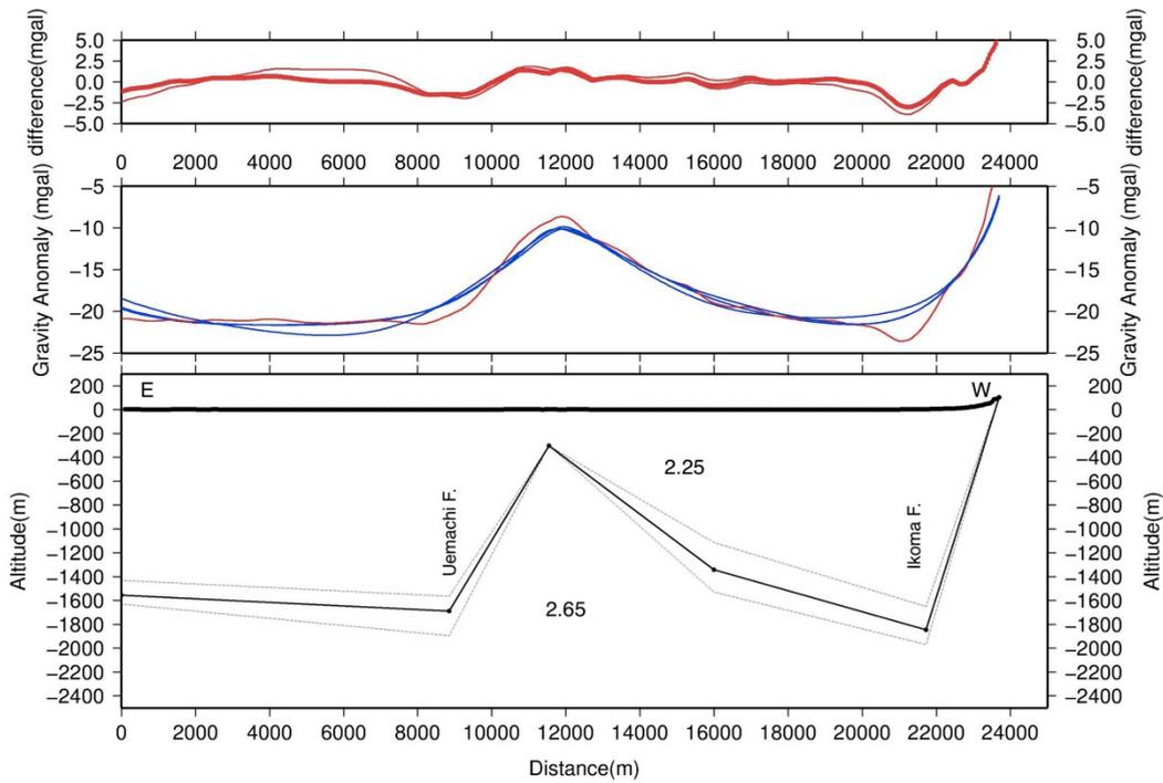
**Figure 3.** Profile of the L3 in Fig. 2. Top: difference between observed and calculated gravity anomaly form the model. Middle: Observed (red line), calculated gravity anomaly (blue line). Bottom: underground model. Numerical values in figures denote the density of the basement (2.65) and sediments (2.25). The dashed lines in the figure are minimum and maximum values during 5 results. The solid line is the average value of 5 results.
