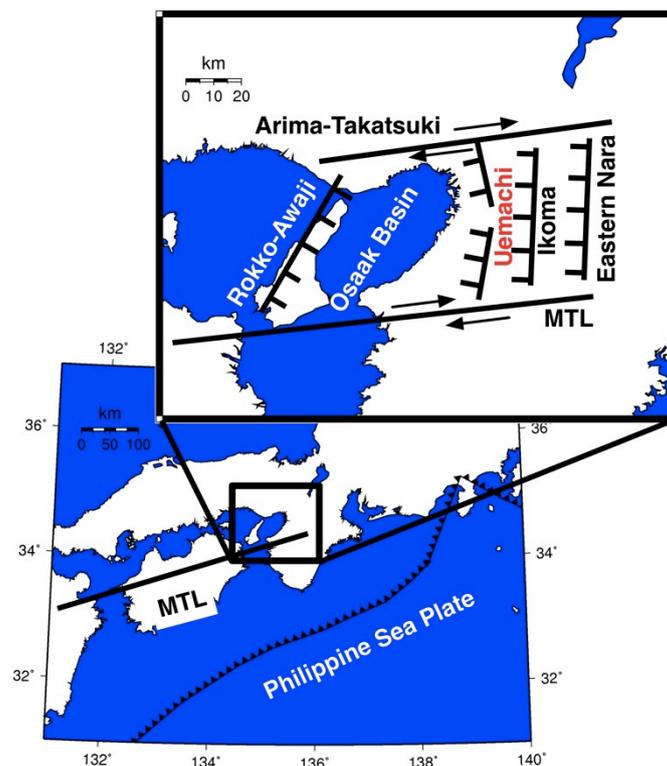
**Figure 1.** Schematic figure of the Osaka basin and surrounding faults. The solid line with the arrow indicates the strike-slip fault. The solid line with the hachure denotes the reverse fault.
