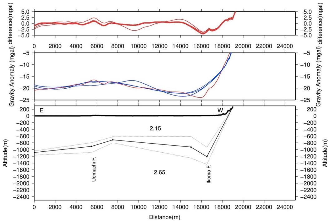
**Figure 4.** Profile of the L4 in Fig. 2. Top: difference between observed and calculated gravity anomaly form the model. Middle: Observed (red line), calculated gravity anomaly (blue line). Bottom: underground model. Numerical values in figures denote the density of the basement (2.65) and sediments (2.15). The dashed lines in the figure are minimum and maximum values during 5 results. The solid line is the average value of 5 results.
