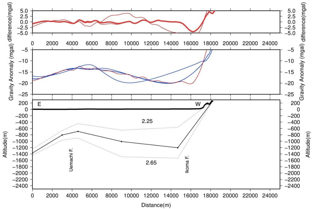
**Figure 5.** Profile of the L5 in Fig. 2. Top: difference between observed and calculated gravity anomaly from the model. Middle: Observed (red line), calculated gravity anomaly (blue line). Bottom: underground model. Numerical values in figures denote the density of the basement (2.65) and sediments (2.25). The dashed lines in the figure are minimum and maximum values during 5 results. The solid line is the average value of 5 results.
