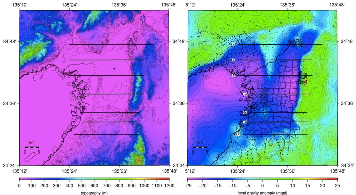
**Figure 2.** Topography (left) and gravity anomaly (right) of the Osaka basin. Left: Contour map of the topography based on 50m digital elevation model published from the Geographical Society of Japan. The contour interval is 5m below 40m and is 50m above 40m. Right: Local gravity anomaly map (Inoue et al., 2000). The contour interval is 2 mgal. The solid circles in the figure show the gravity station. The thick solid lines denote the investigated profiles in this study.
