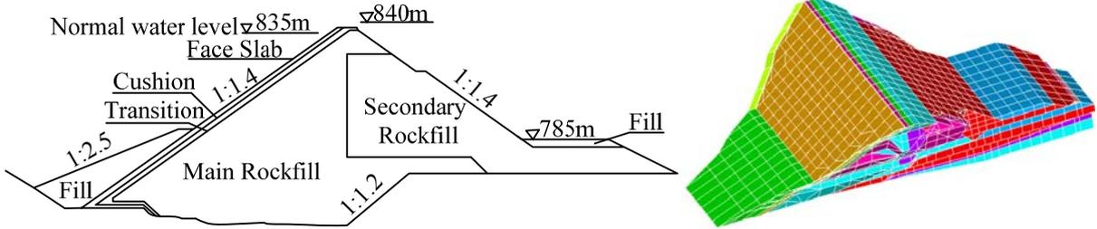
Figure 5. Typical cross section and three dimensional mesh of Yayangshan
