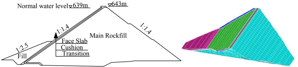
Figure 6. Typical cross section and three dimensional mesh of Longma
