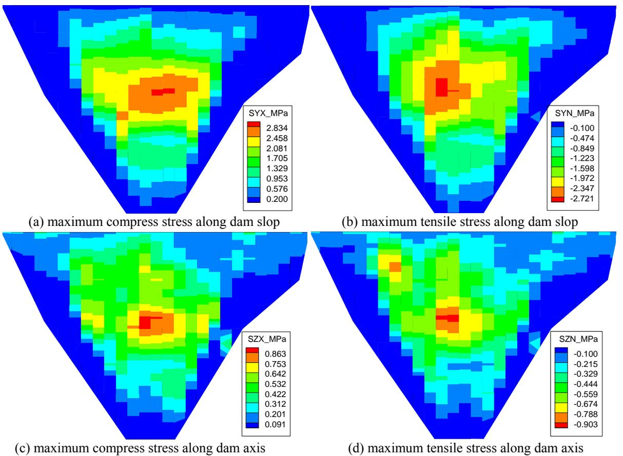
**Figure 13.** Maximum stress response of face slab distribution of Longma
