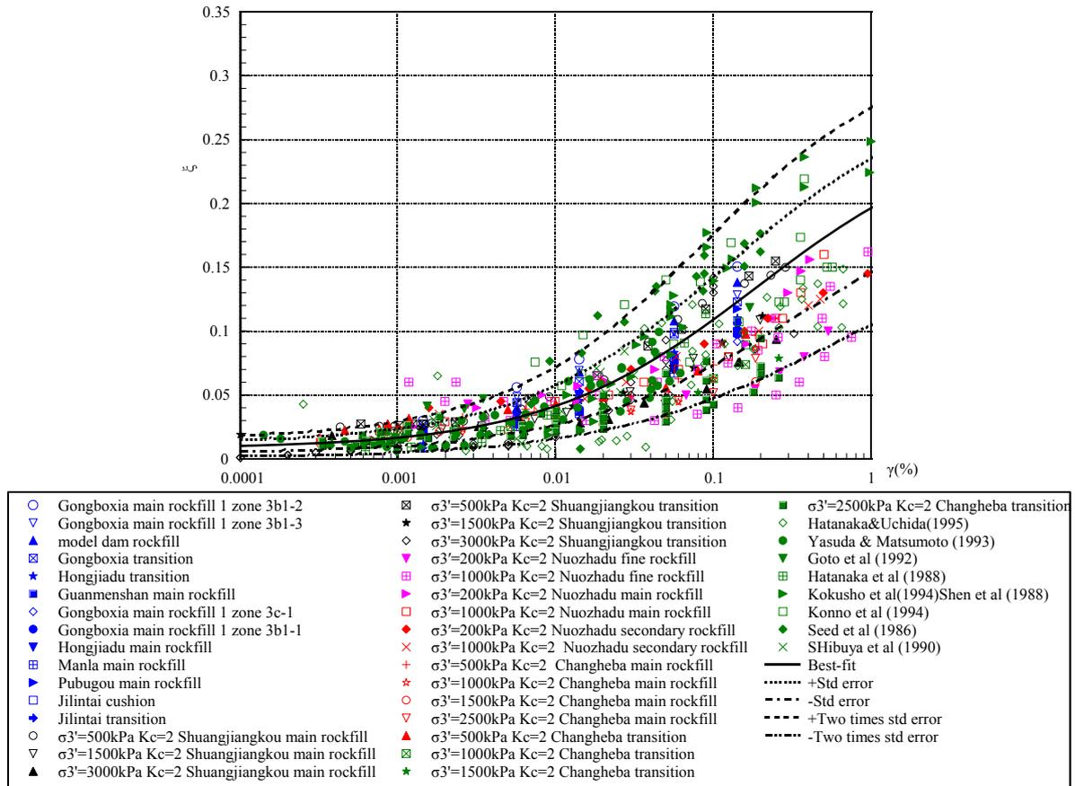
**Figure 2.** Data points defining  $\xi$  versus  $\gamma$  relationships for 35 kinds of rockfills based on testing along with the best-fit curve,  $\pm$  one standard division curves and two times standard division curves.
