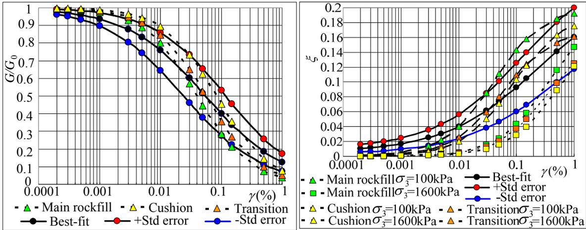
Figure 8. The  $G/G_0 \sim \gamma$  curve and  $\xi \sim \gamma$  curve of the soil used in Longma
