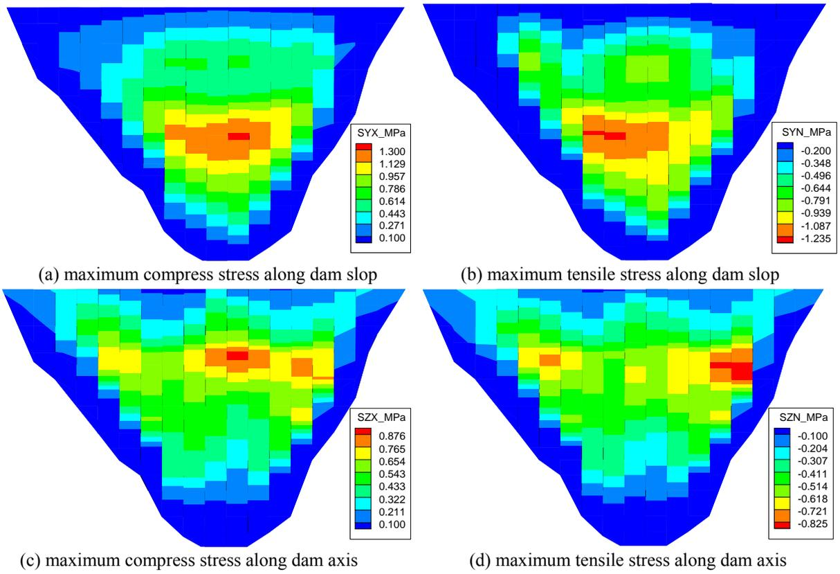
**Figure 13.** Maximum stress response of face slab distribution of Yangyashan
