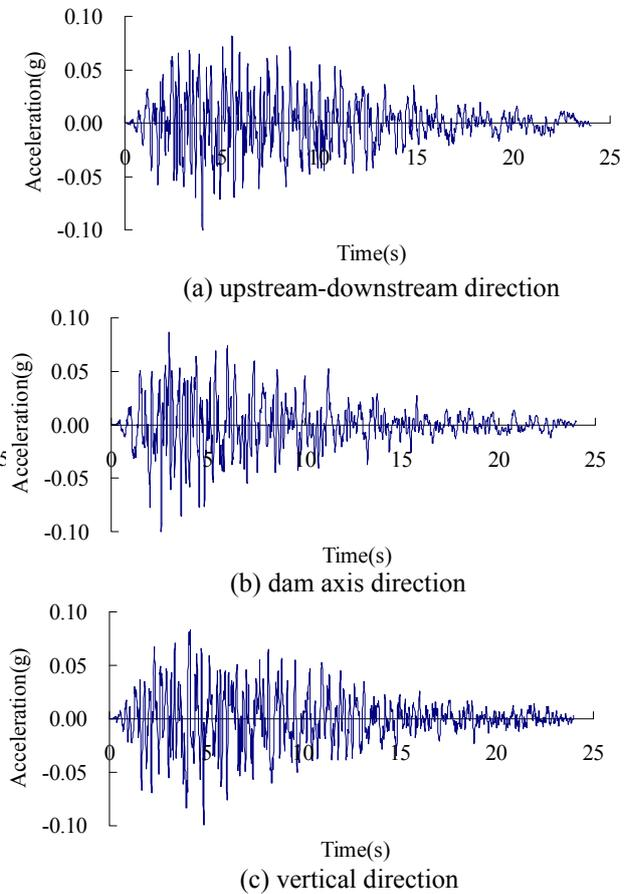
Figure 10. Design earthquake of Longma
