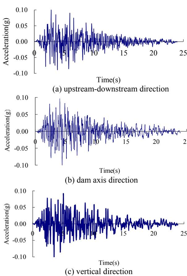
Figure 9. Design earthquake of Yangyashan
