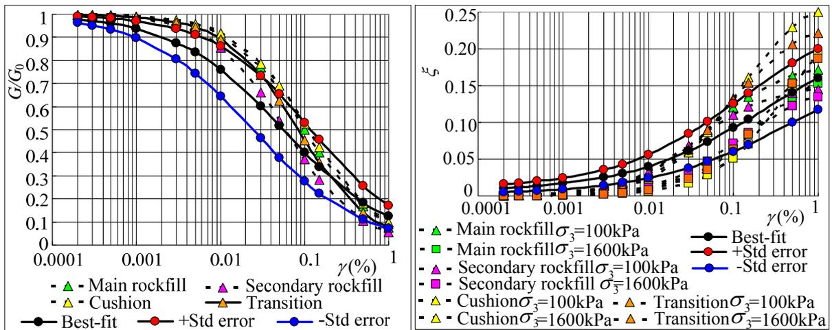
**Figure 7.** The  $G/G_0 \sim \gamma$  curve and  $\xi \sim \gamma$  curve of the soil used in Yayangshan
