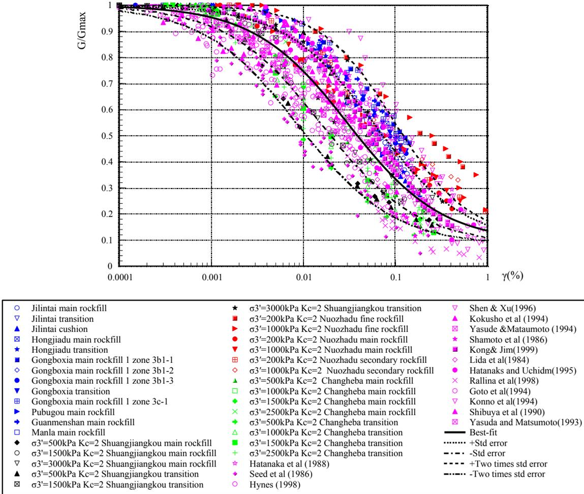
**Figure 1.** Data points defining  $G/G_0$  versus  $\gamma$  relationships for 35 kinds of rockfills based on testing along with the best-fit curve,  $\pm$  one standard division curves and two times standard division curves.
