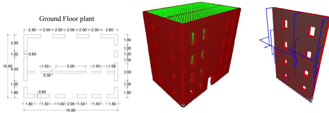
**Figure 5.** Case study building (on the left and in the middle) and the isostatic loading system (on the right)
