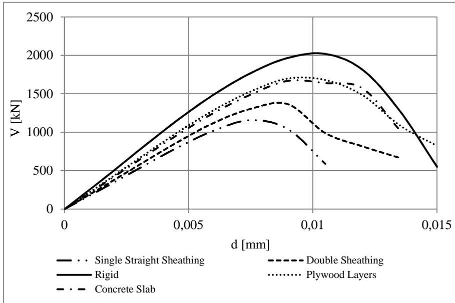
**Figure 11.** Capacity curves (2 m of additional eccentricity to the mass centre)
