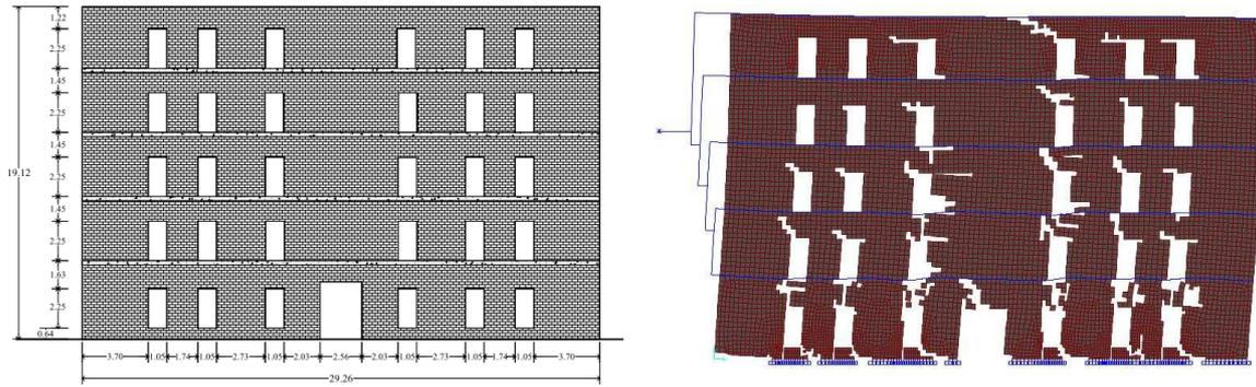
**Figure 3.** Via Martoglio wall – Unloaded condition (on the left), ultimate condition (on the right)
