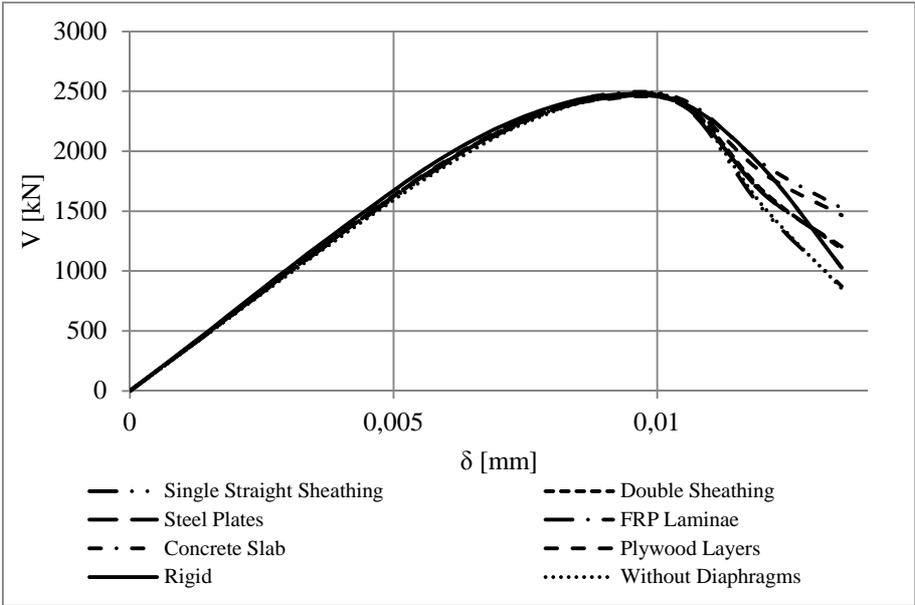
Figure 9. Capacity curves (different floor-typologies)
