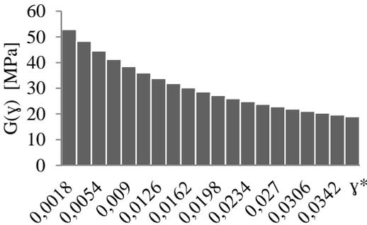
**Figure 6.** Equivalent shear stiffness (Double sheathing)
