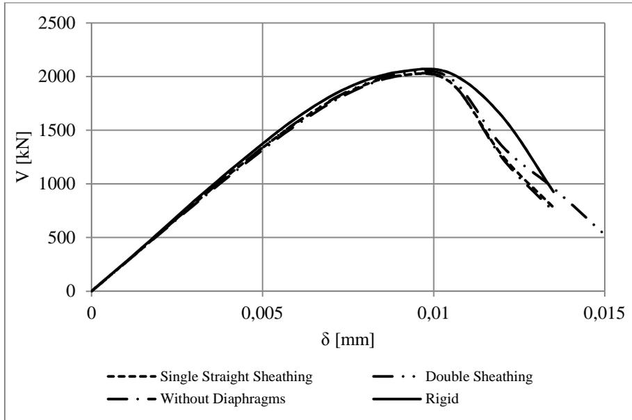
**Figure 10.** Capacity curves (North wall with halved thickness)
