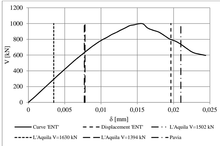
**Figure 4.** Capacity curve of the Via Martoglio wall
