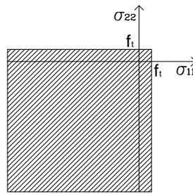
**Figure 1.** Failure criterion in terms of principal stresses ( $f_t$  = tensile strength of masonry)
