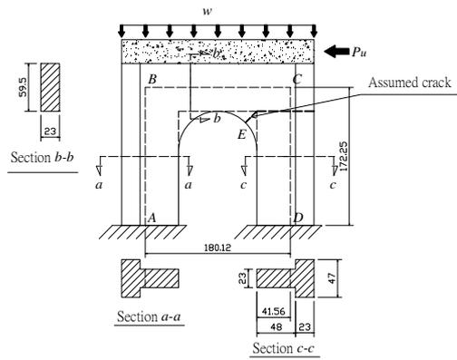
**Figure 5.** Assumed initial crack position of brick arch specimen (unit:cm)
