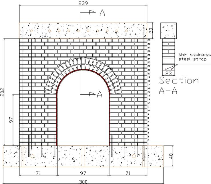
**Figure 1.** Brick arch specimen, 2 thin stainless steel straps are imbedded into the intrados face of the brick arch (specimens WS1, WR1 and WR2)
