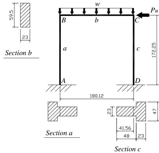
**Figure 6.** Analysis model for brick arch specimen (unit:cm)
