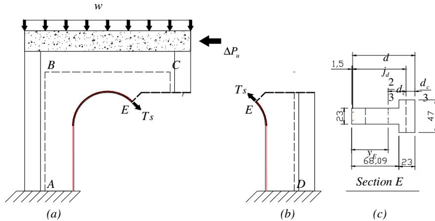
**Figure 8.** Free body on joint C of brick arch specimen
