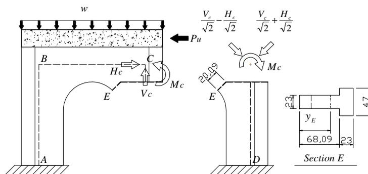
**Figure 7.** Free body on joint C of brick arch specimen
