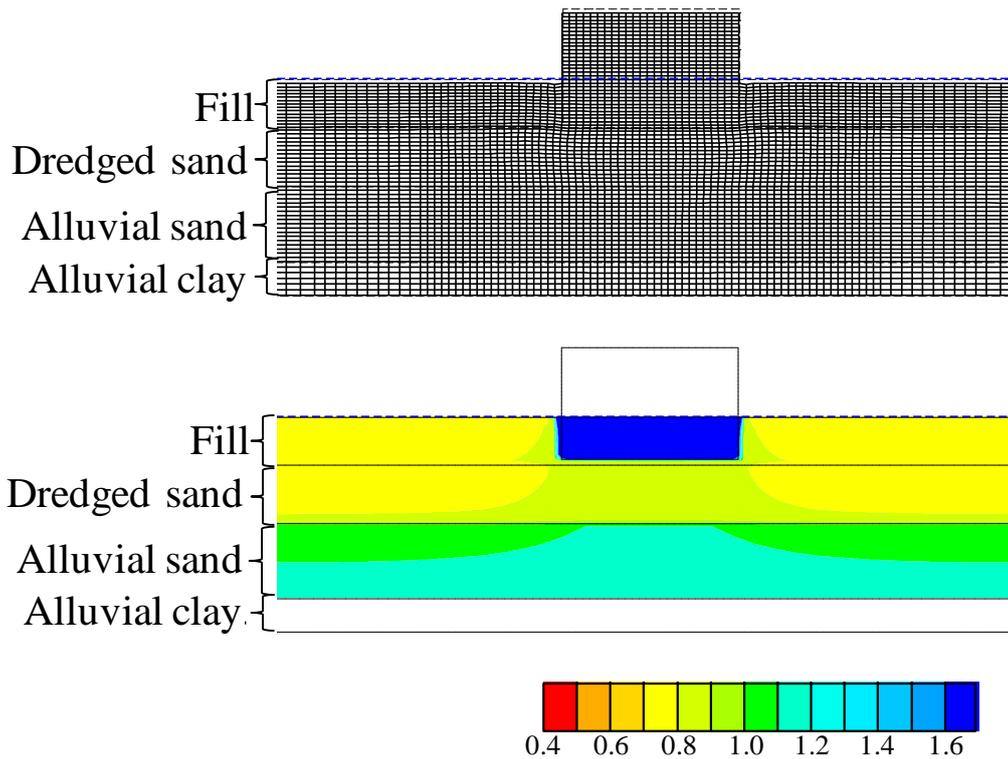
Figure 11. Deformation of basic case (WL= 0m, Compacted up to the depth of 3.0 m)
