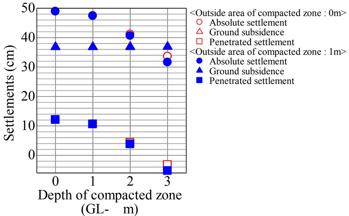
Figure 12. Relationship between depth of compacted zone and settlements
