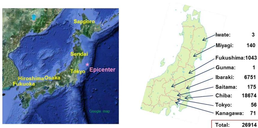
**Figure 1.** Numbers of the damaged houses due to liquefaction in each prefecture during the 2011 Tohoku-Pacific Ocean earthquake
