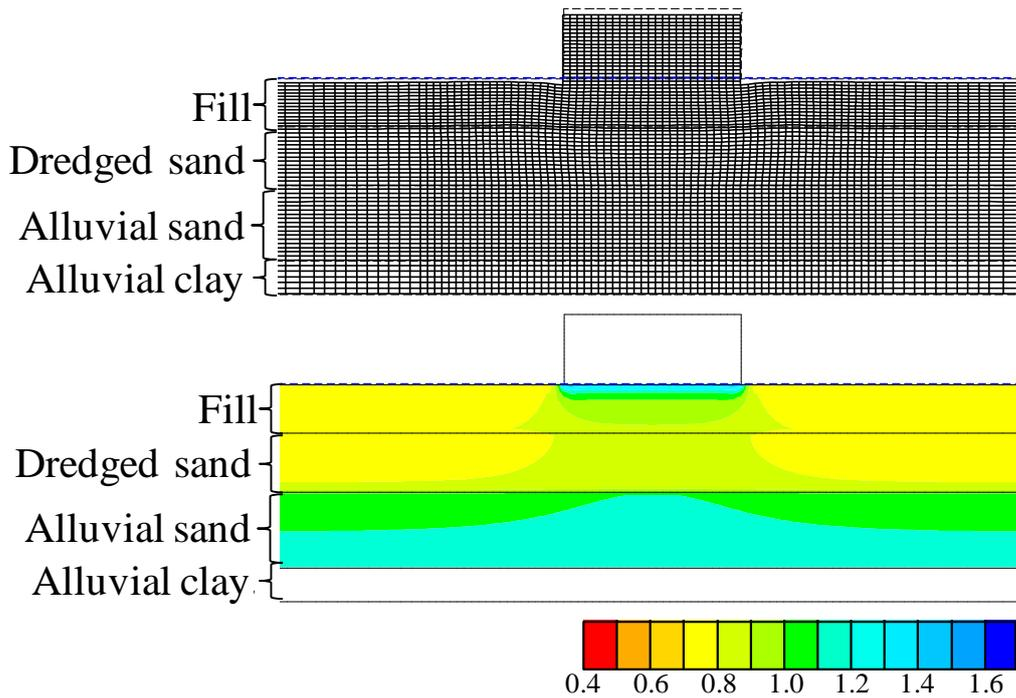
Figure 9. Deformation of basic case (WL= 0m, without compaction)
