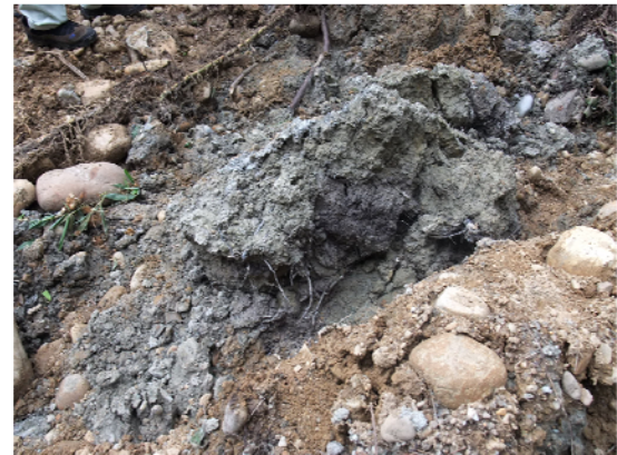
Figure 3. Weathered mudstones observed at the toe of the failed slope
