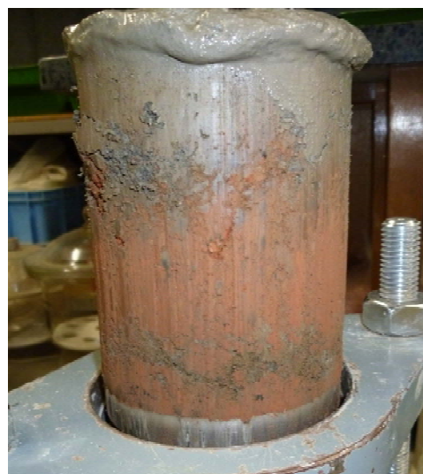
Figure 9. A specimen after 5 cycles of slaking
