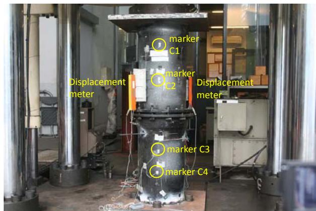
**Figure 6.** The displacement meters and NDI markers from C1 to C4
