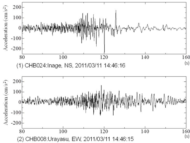
**Figure 8.** Comparison of accelerographs recorded at K-NET Inage and Urayasu
