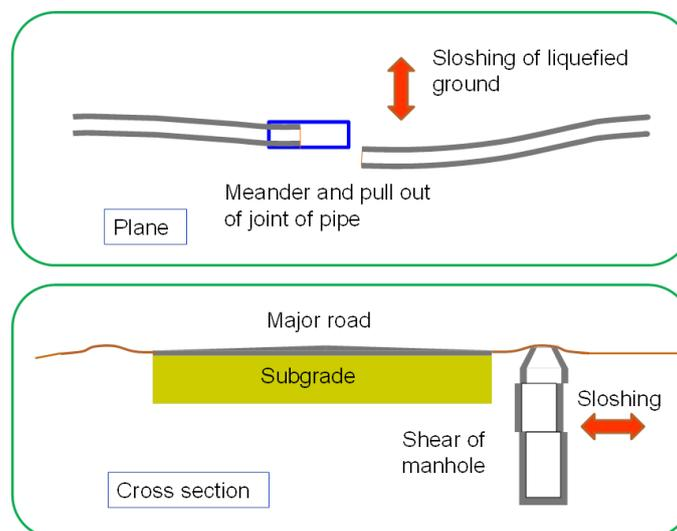
**Figure 15.** Unique damage to sewage manholes and pipes
