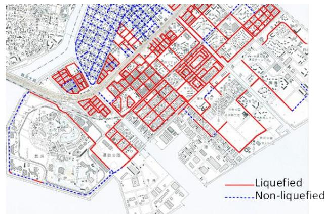
Figure 4. Method to judge liquefied and non-liquefied zones
