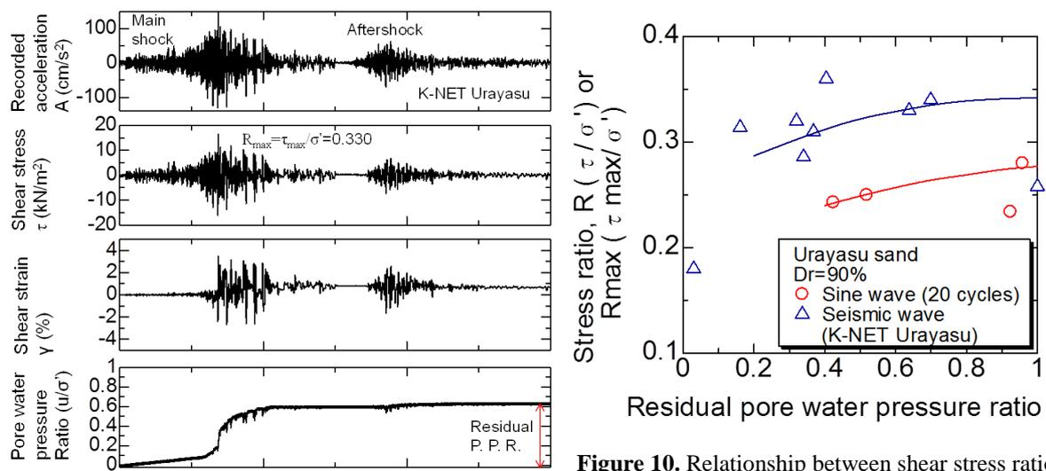
**Figure 9.** Time histories of shear stress, shear strain and excess pore water pressure
