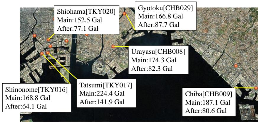
**Figure 7.** Comparison of accelerations during main and aftershocks by K-NET
