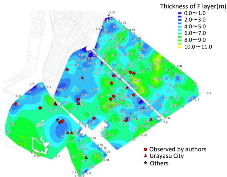
**Figure 14.** Heaved footways or alleys in Urayasu City together with contour lines of the thickness of the F layer under the ground water table (Contour lines are quoted from research materials (2011))
