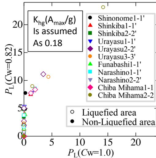
Figure 12. Effect of  $C_w$  on  $P_L$
