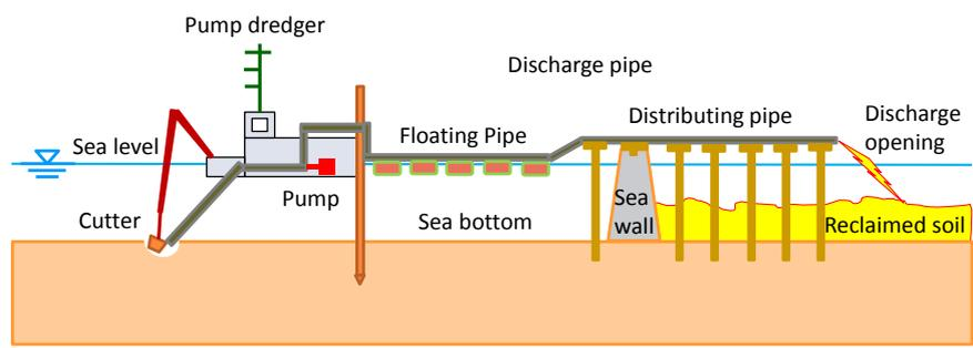
**Figure 3.** Process of dredging work
