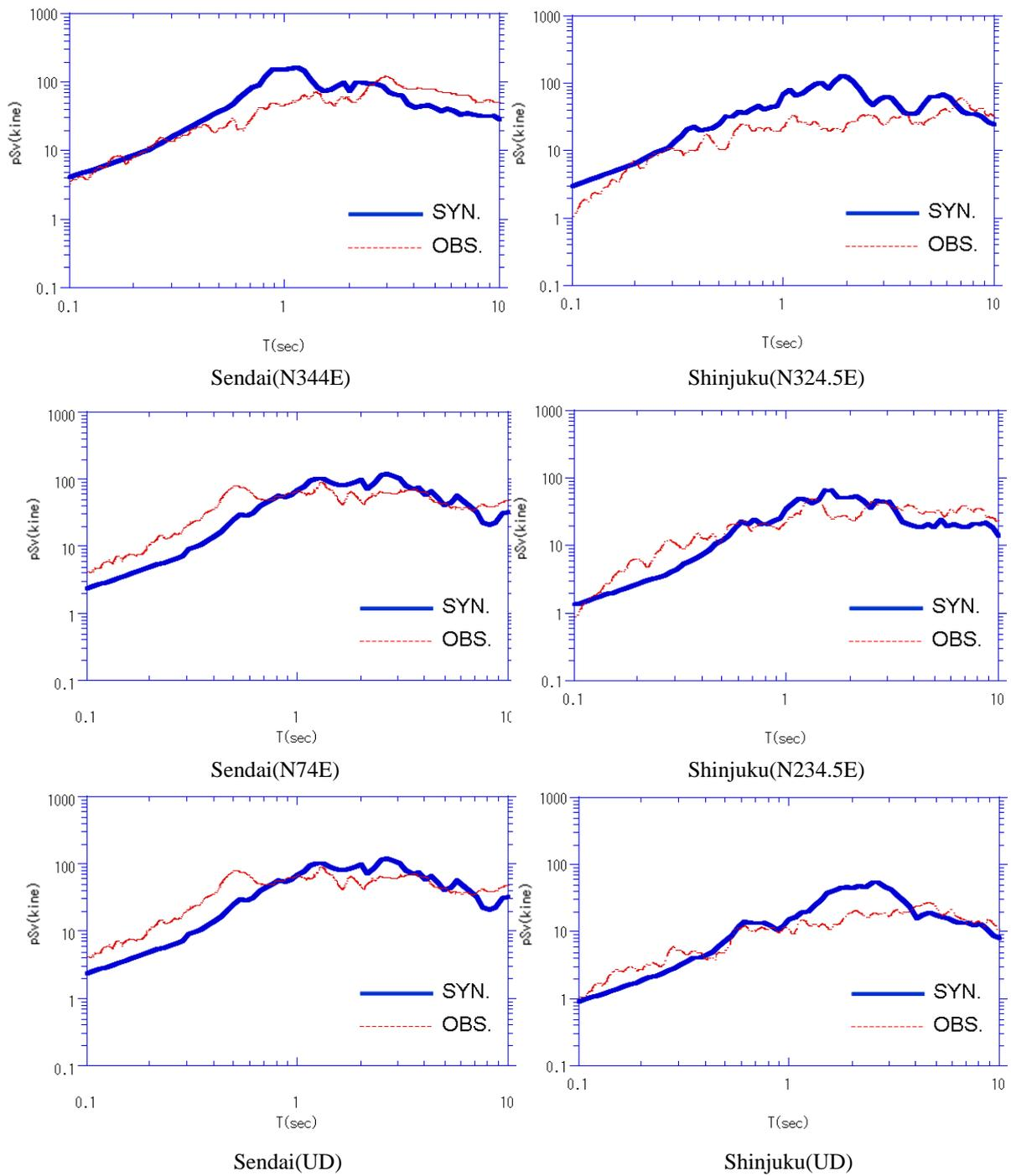
**Figure 5.3.** Comparison of observed and synthetic velocity response spectra for Sendai and Shinjuku site (damping ratio  $h = 5\%$ )
