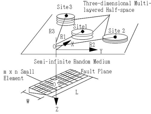
**Figure 4.** Geometric relation between causative fault and sites
