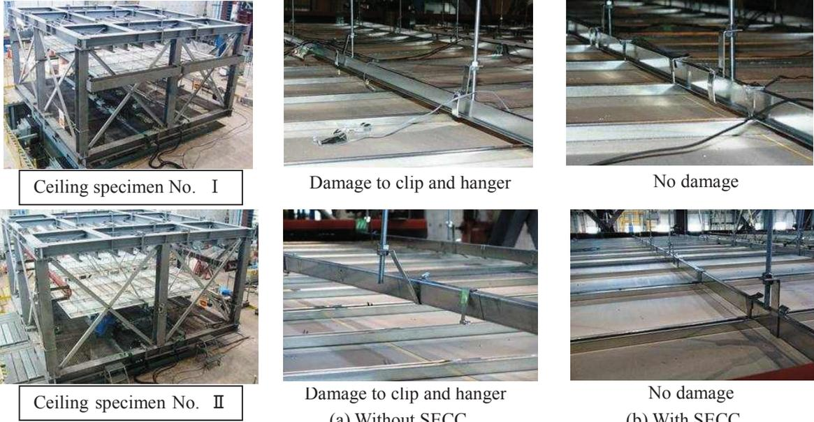
**Photograph 4.** Examples of damage to metal furring suspended ceiling with and without SECC
