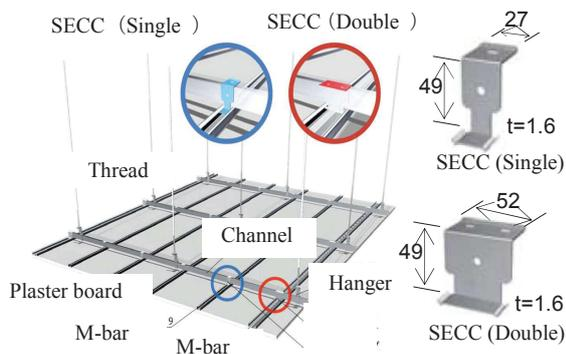
**Figure 5.** Schematic of SECC (unit: mm)
