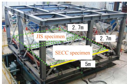
**Photograph 3.** Test frame and the suspended ceiling specimen mounted on a shaking table
