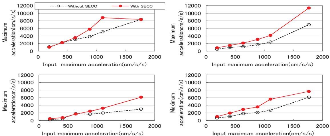
**Figure 9.** Relationships between input vertical motion and maximum vertical acceleration response on the plasterboard of the metal furring suspended ceiling with and without the SECC
