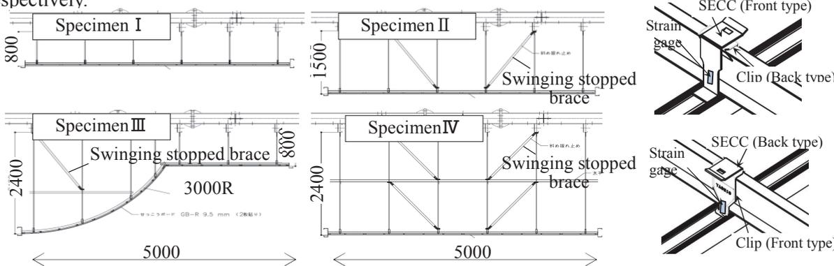
**Figure 6.** Elevation of the metal furring suspended ceiling specimens (unit: mm)
