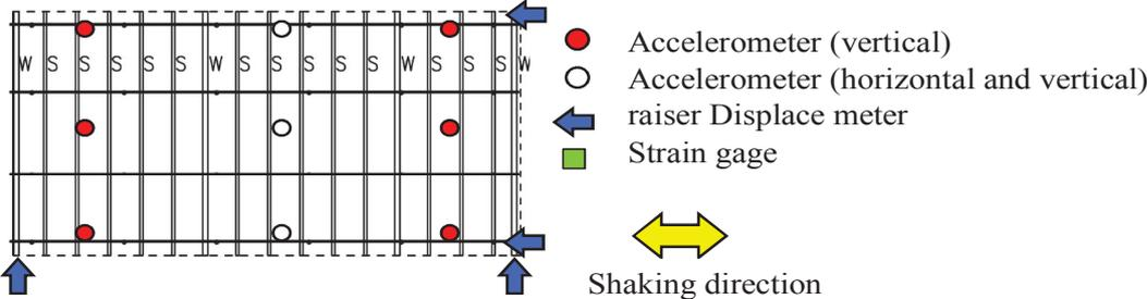
**Figure 7.** Locations of accelerometers on the suspended ceiling and transducers at the base of the frame
