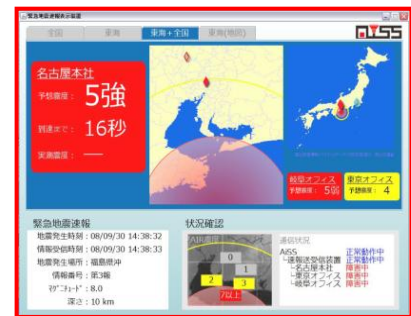
Photo 3.2. (1) EEW terminal system installed in the user's office, (2) FTE alarm display (monitor, flash light and alarm sound), (3) monitor display of PC: propagating P- and S-wave front, estimated intensity, time until arriving strong motion, etc.
