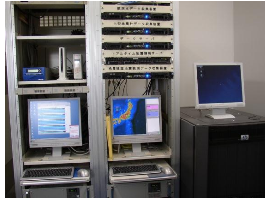
Photo 3.1. Servers for receiving and delivering EEW in the DPREC office
