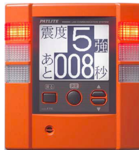
Photo 3.2. (1) EEW terminal system installed in the user's office, (2) FTE alarm display (monitor, flash light and alarm sound), (3) monitor display of PC: propagating P- and S-wave front, estimated intensity, time until arriving strong motion, etc.
