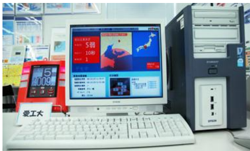
Photo 3.2. (1) EEW terminal system installed in the user's office, (2) FTE alarm display (monitor, flash light and alarm sound), (3) monitor display of PC: propagating P- and S-wave front, estimated intensity, time until arriving strong motion, etc.
