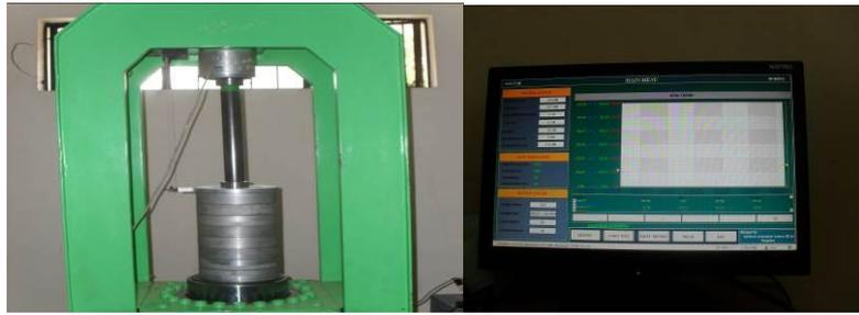
Figure 1. Columns being tested under Cyclic Loading Equipment
