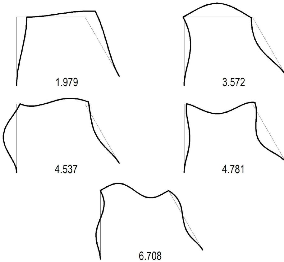
**Figure 4.6.** The first 5 modes of the sloping-frame with  $\theta = 60^\circ$
