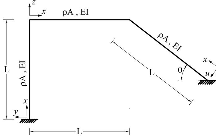
Figure 2.1. The semi-inclined frame under study
