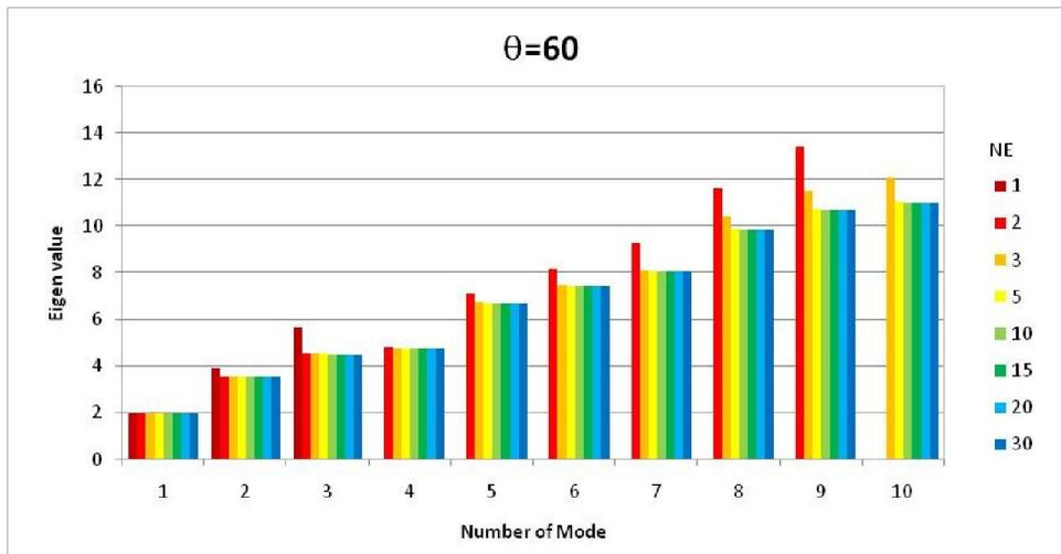
**Figure 4.4.** Effect of the number of elements (NE) on the accuracy of the modified finite element response  $\theta = 60^\circ$
