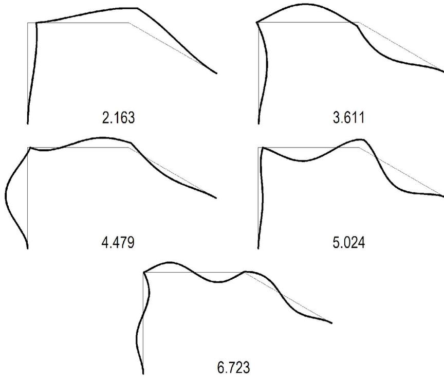
**Figure 4.5.** The first 5 modes of the sloping-frame with  $\theta = 30^\circ$
