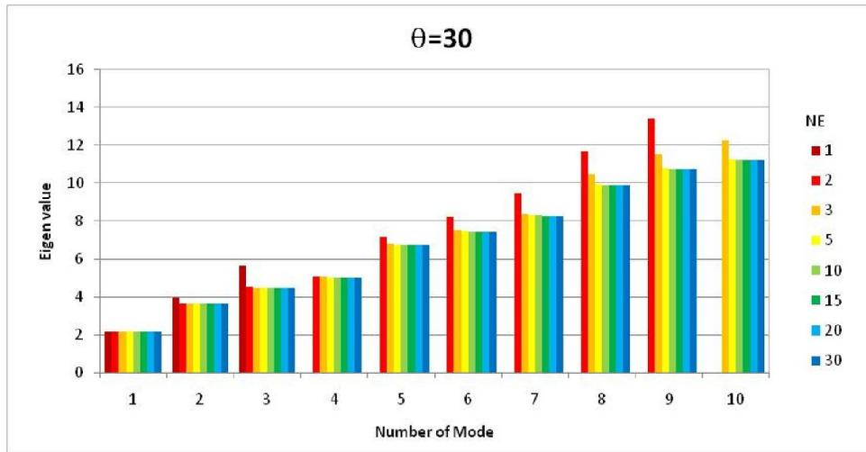
**Figure 4.3.** Effect of the number of elements (NE) on the accuracy of the modified finite element response  $\theta = 30^\circ$
