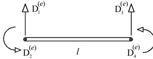
Figure 3.1. The bending element
