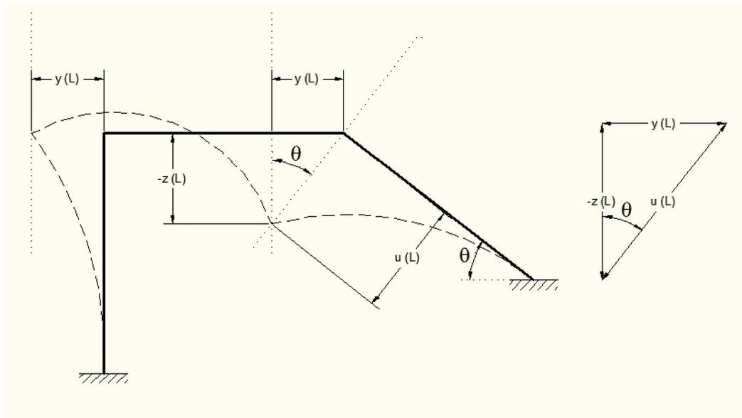
**Figure 2.2.** Bending deformation diagram based on neglecting of the axial deformation
