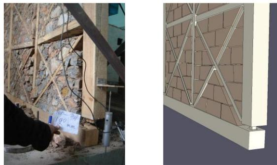
**Figure 15.** Wall panel deformation at 120mm top displacement
