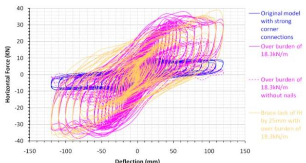
**Figure 22.** Hysteresis loop comparisons at 18.3kN/m
