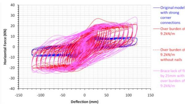
**Figure 21.** Hysteresis loop comparisons at 9.2kN/m
