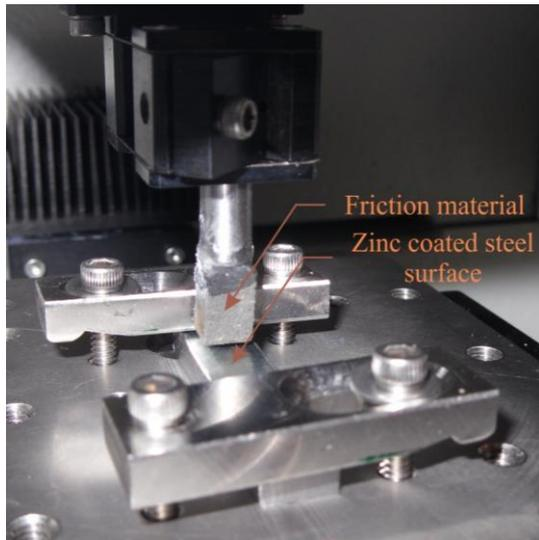
**Photo 2.** Experimental test setup
