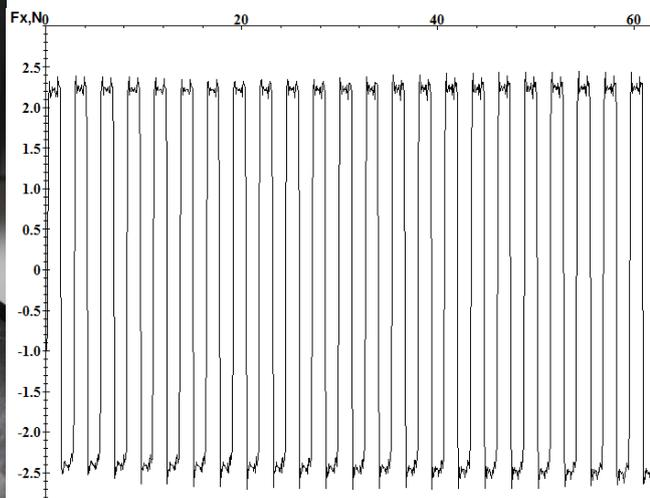
**Figure 2.** Friction force variation for a 12 mm/sec test speed
