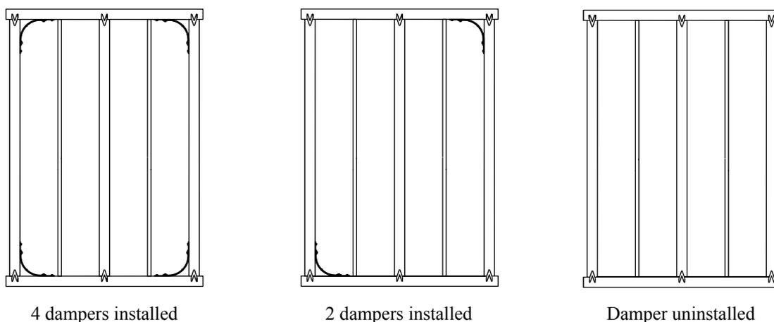
Figure 4. 1. Test frame types of bearing wall
