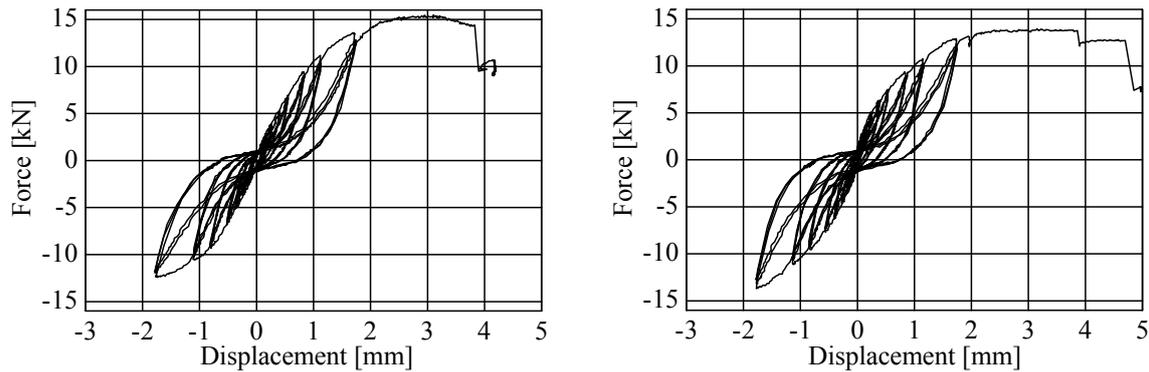
**Figure 5. 1.** Force-displacement curves of the test frame with wood brace
