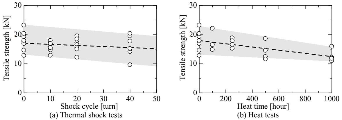
**Figure 3.1.** Adhesive strength of the viscoelastic material
