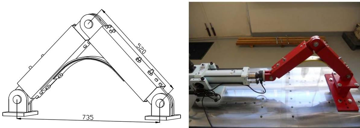
**Figure 3. 2.** L-shaped crank mechanism
