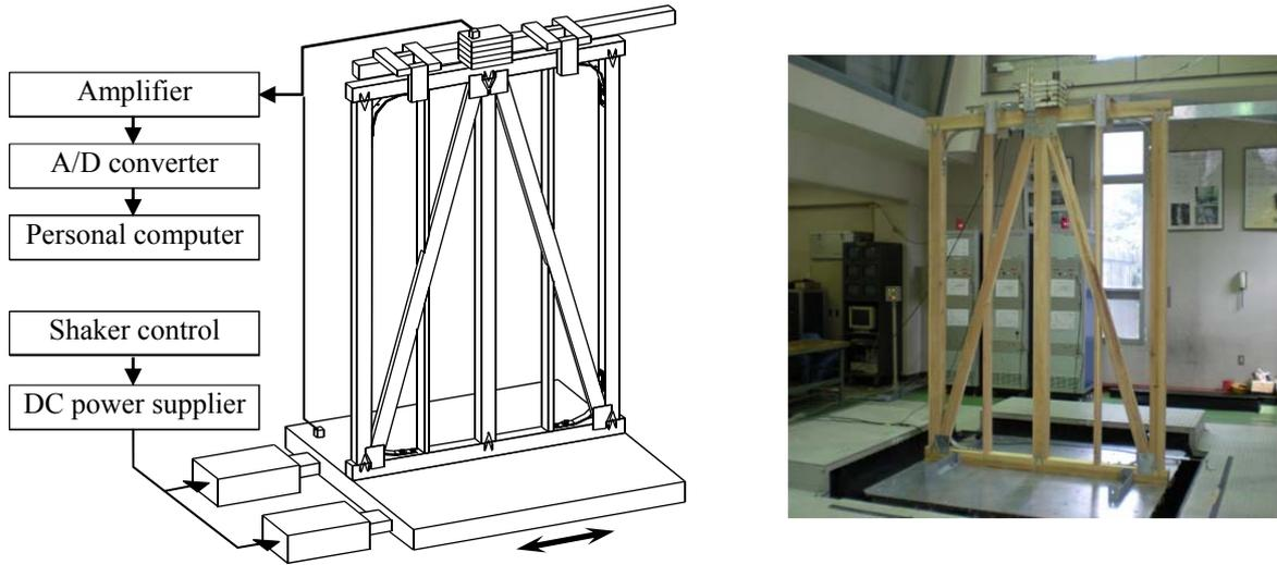
**Figure 4. 2.** Shaking test setup
