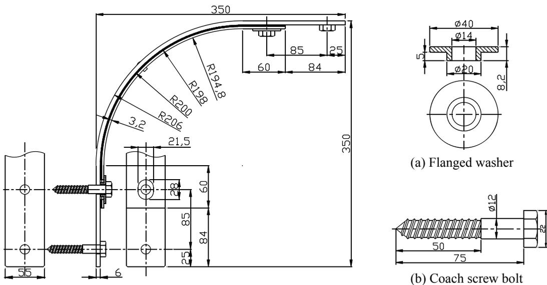
**Figure 2. 1.** Design diagram of arc shaped spring damper
