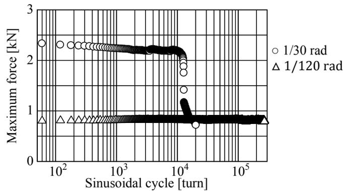
**Figure 3. 5.** Durability of the damper
