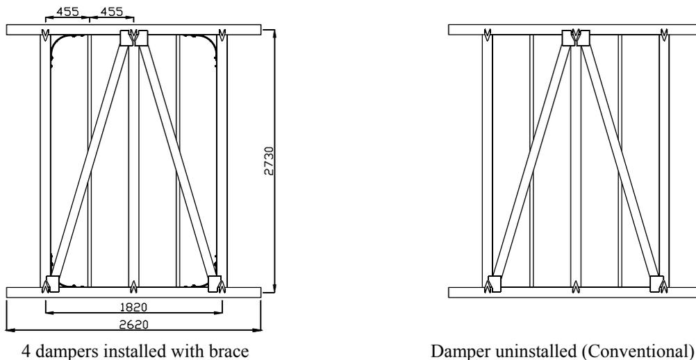
**Figure 4. 1.** Test frame types of bearing wall
