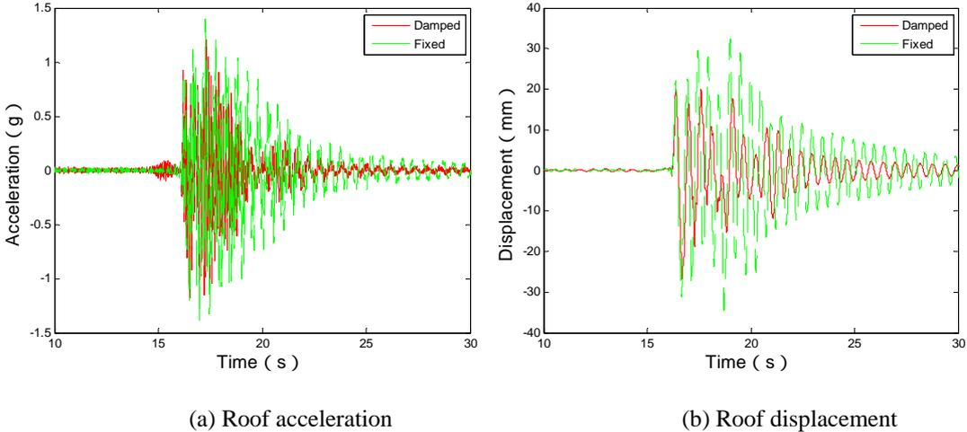
**Figure 6.** Time history responses of test structure with fixed and damped outrigger under El Centro 0.6g motion
