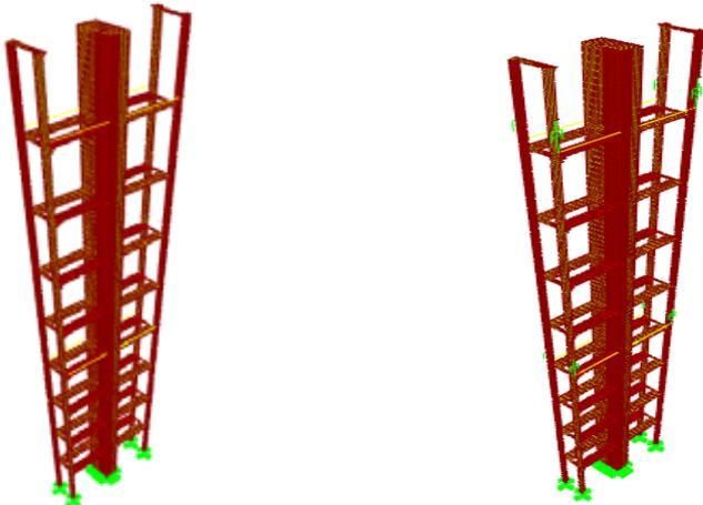
(a) Fixed-Outrigger model                      (b) Damped-Outrigger model
