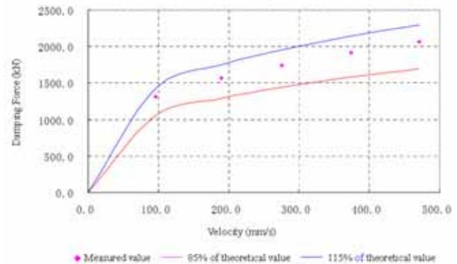
**Figure 2.** Force-Velocity relationship of viscous damper
