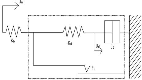
Figure 7. Modified Analytic model of viscous damper
