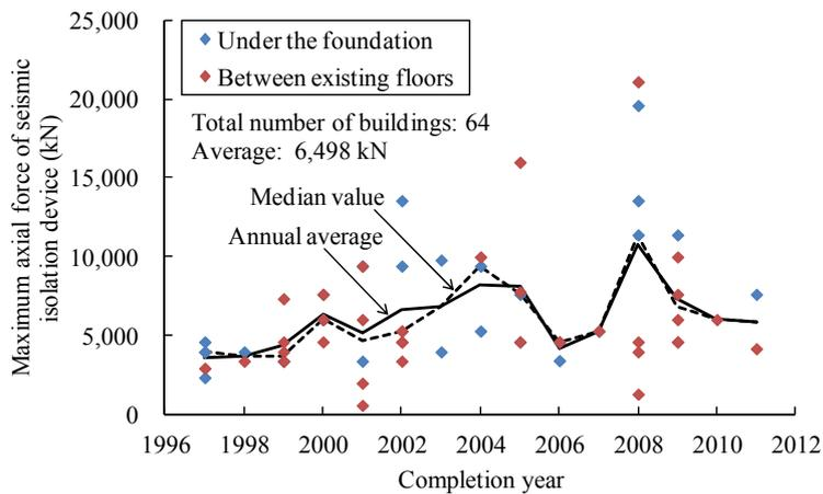
Figure 2.4.3. Relationship between completion year and maximum axial force of seismic isolation devices
