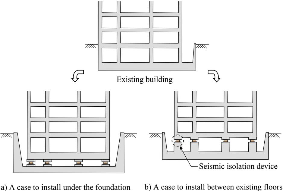
Figure 2.3.1. Location of seismic isolation layer
