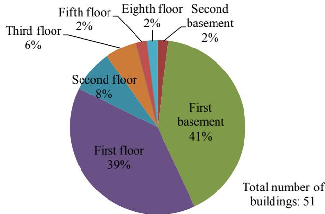
**Figure 2.3.3.** Ratio of floors of seismic isolation layer in the cases to install between existing floors
