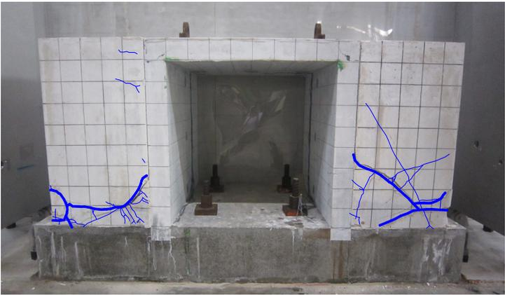
Figure 6. Damage condition of improvement body
