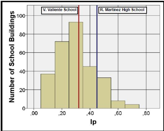
**Figure 4.** Prioritization index (Ip) for the inspected 294 schools as compared with the collapsed schools.
