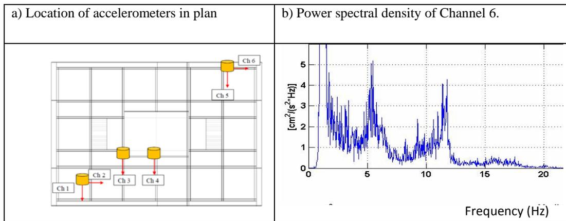
**Figure 5.** Determination of dynamic properties for low intensity motion in School N° 5.
