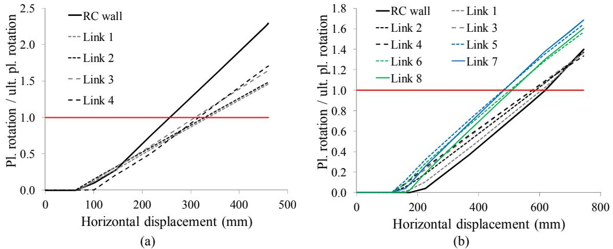
Figure 4. Plastic rotations for: (a) 4-storey case, (b) 8-storey case.
