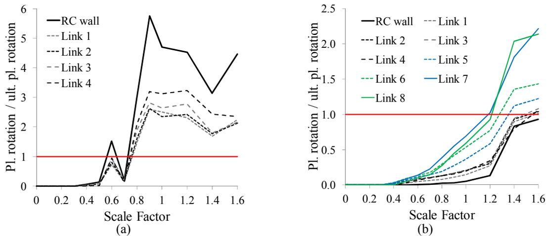
**Figure 4.** Evolution of plastic rotations (IDA average values) for: (a) the 4-storey case, (b) 8-storey case.
