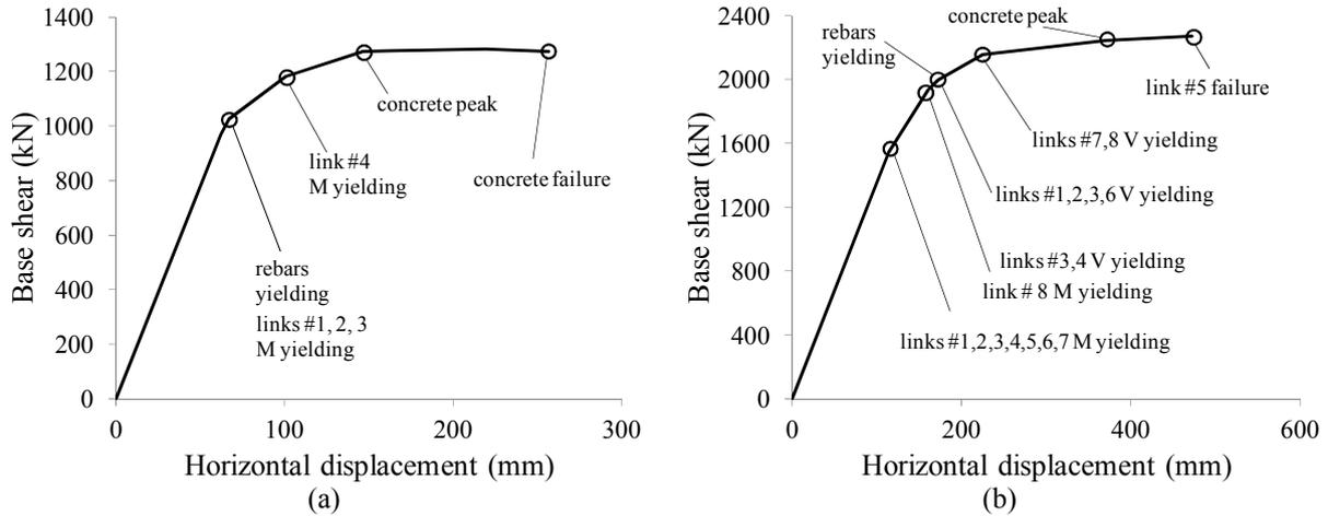
Figure 4. Pushover curves for: (a) 4-storey case, (b) 8-storey case.
