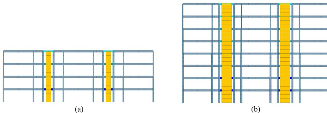
**Figure 3.** Innovative HCSW system with additional columns: (a) 4-storey case, (b) 8-storey case.
