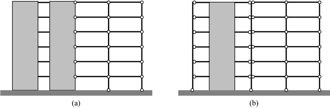
**Figure 1.** Examples of: (a) conventional hybrid coupled shear wall system, (b) innovative hybrid coupled shear wall system, both connected to a gravity-resisting steel frame with pinned beam-to-column joints.
