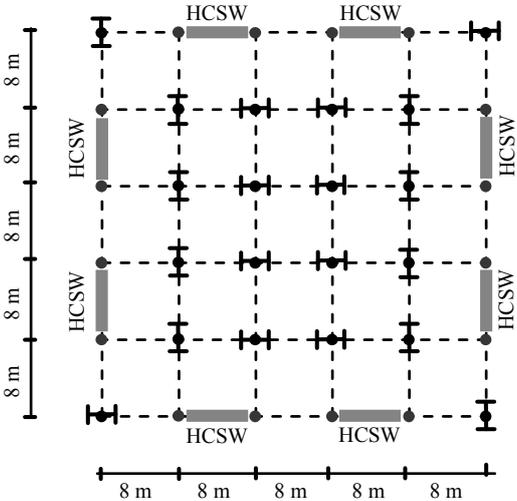
**Figure 2.** Floor geometry of the benchmark structures with positions of the HCSW systems.
