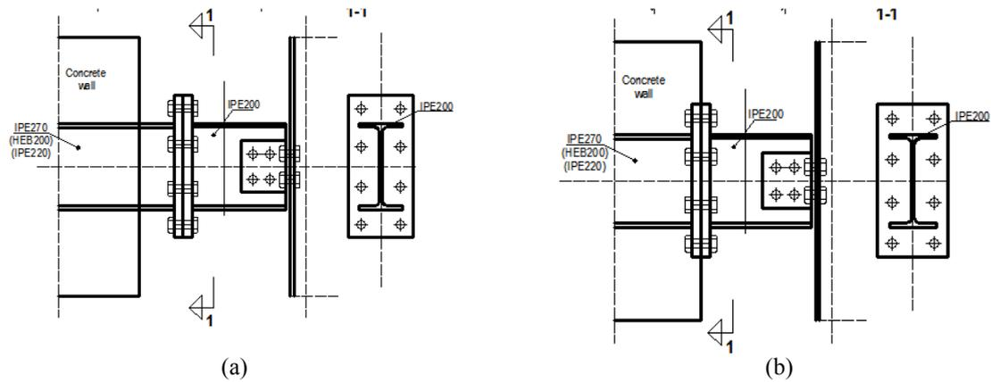
**Figure 6.** Link splice typology 1 (a) and typology 2 (b).
