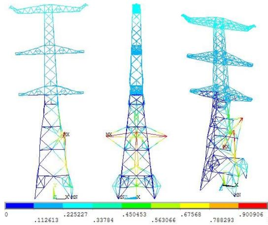
**Figure 4.** The first buckling mode shape
