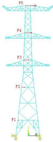
**Figure 2.** The horizontal load pattern
