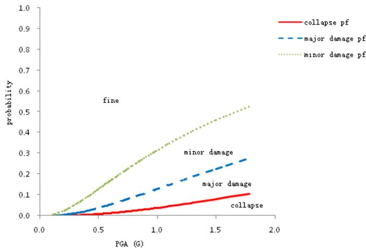
**Figure 13.** The seismic fragility curve of the transmission tower
