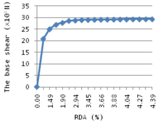
**Figure 5.** The base shear force versus the top rotation angle
