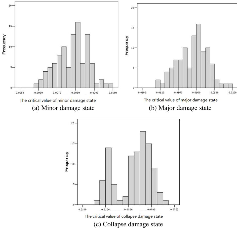
**Figure 7.** Statistical histogram of the displacement limits (rad)
