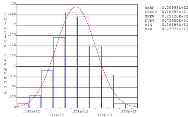
**Figure 6.** The sampling distribution of elastic modulus of steel
