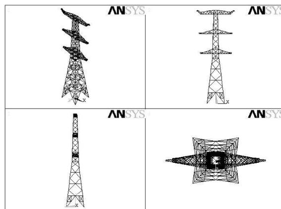
**Figure 1.** The finite element model of transmission tower
