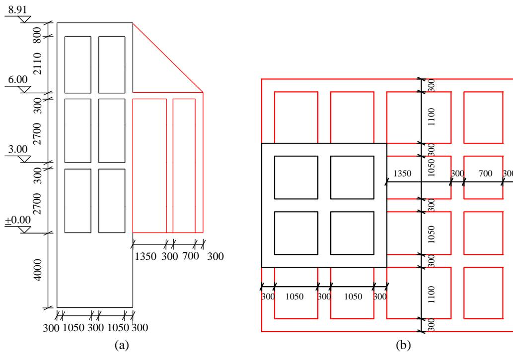
**Figure 2.** The dynamic machine foundation after strengthening where the figures are in unit of mm. (a) The
