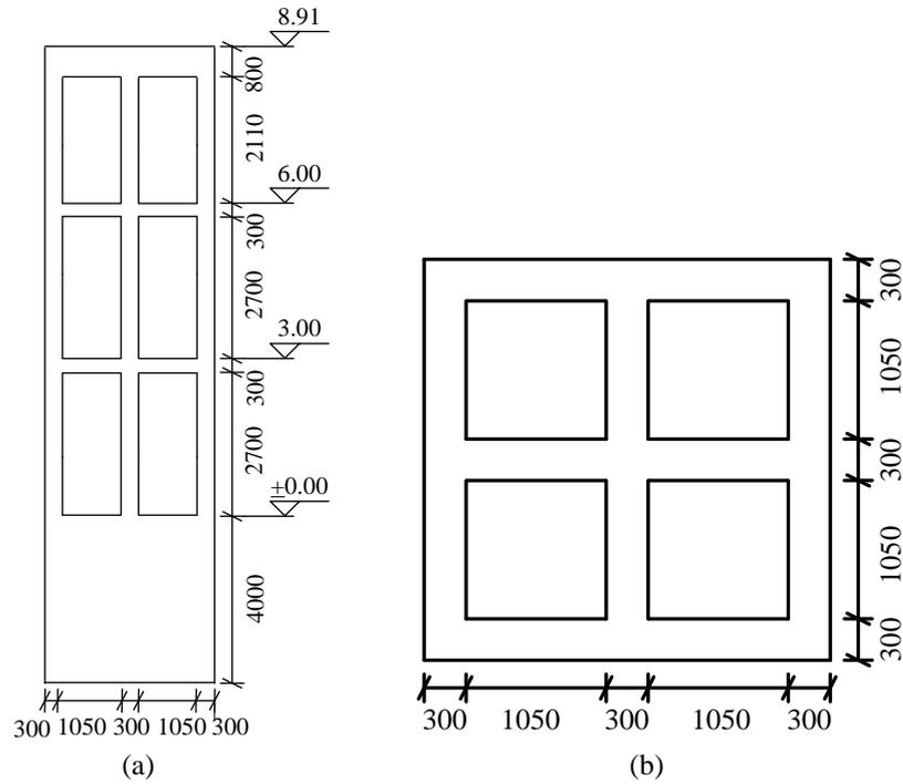
**Figure 1.** The dynamic machine foundation before strengthening where the figures are in unit of mm. (a) The sectional view of the foundation. (b) The shear-wall distribution of the foundation.
