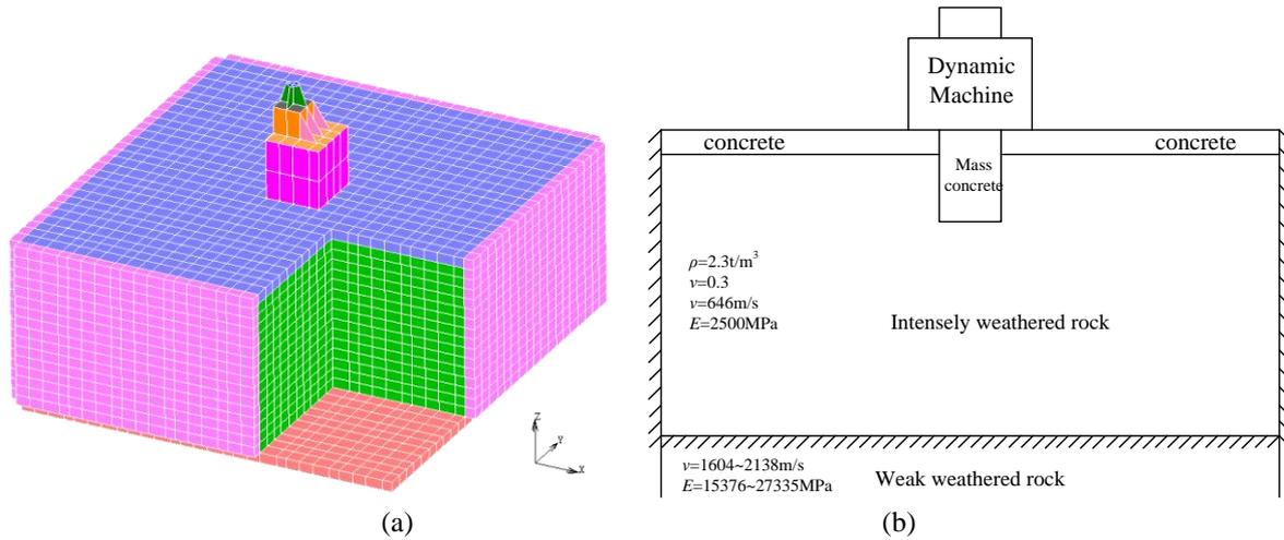
**Figure 7.** The FEA analysis model considering soil-structure interaction. (a) The model of soil-foundation interaction. (b) The properties of the soil layers.
