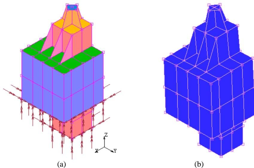
**Figure 5.** The analysis model and result of foundation considering the connection between wall and ground. (a) The analysis model. (b) The fundamental modal and frequency ( $f_1=29.84\text{Hz}$ ) of foundation.
