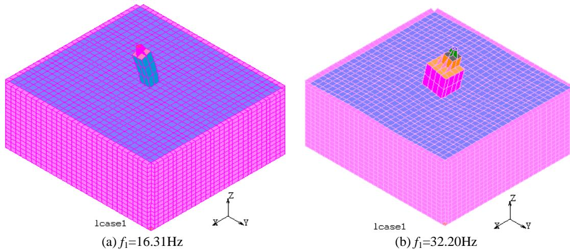
**Figure 8.** The fundamental modal and frequency of foundation considering soil-structure interaction. (a) The foundation before strengthening. (b) The foundation after strengthening.
