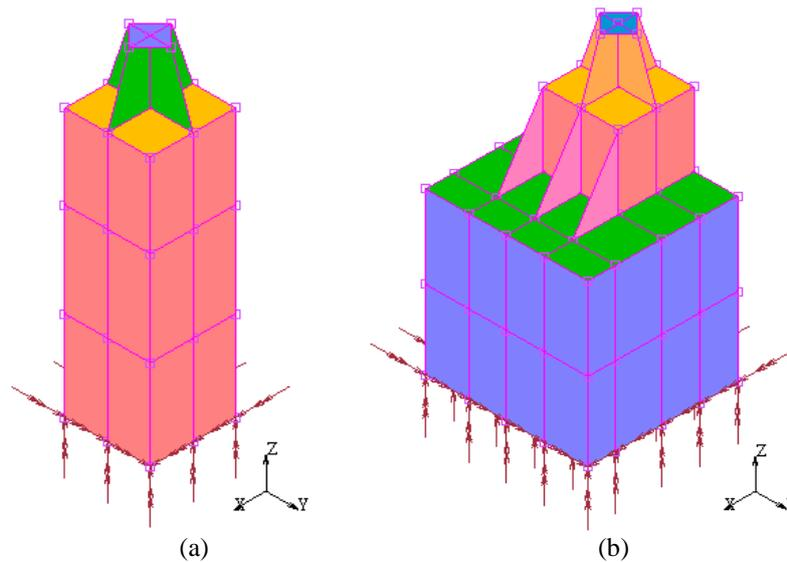
**Figure 3.** The FEA analysis models of foundation based on the assumption of rigid soil. (a) The foundation before strengthening. (b) The foundation after strengthening.
