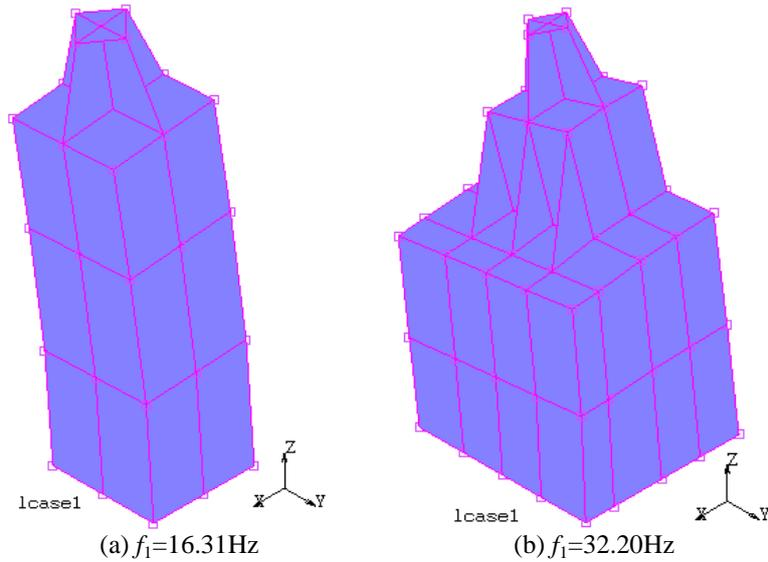
**Figure 4.** The fundamental modal and frequency of foundation based on the assumption of rigid soil. (a) The foundation before strengthening. (b) The foundation after strengthening.
