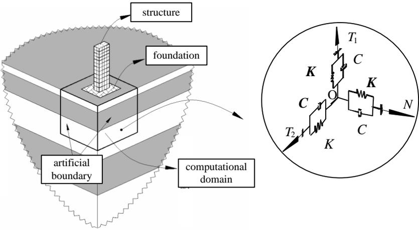
**Figure 6.** The model of 3D viscous-spring artificial boundary
