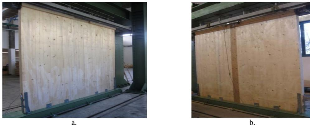
**Figure 3.2.** Experimental setup of full-scale X-Lam wall panels subjected to horizontal load - single wall (left, a.) and coupled wall with LVL spline vertical joint (right, b.)
