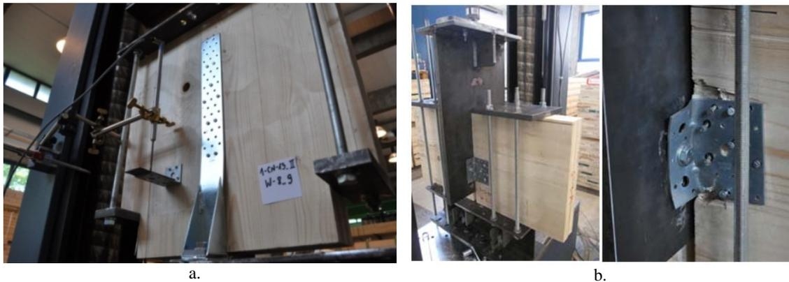
**Figure 3.1.** Experimental setup of hold-down loaded in tension (left a.); angle bracket loaded in shear (right b.)
