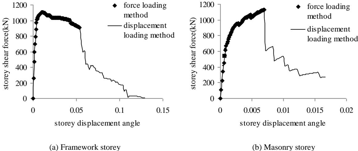
**Figure 4.1.** Shear force-storey displacement angle curves of different storeys of the standard model
