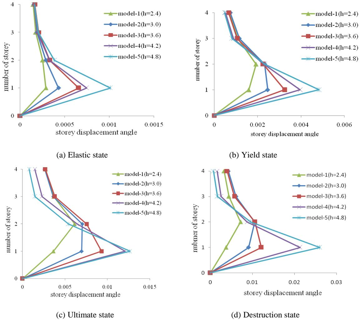
**Figure 4.3.** Storey displacement angle of the models in different states under uniform load
