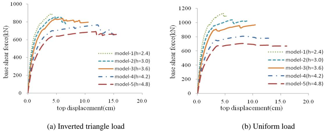
**Figure 4.2.** Base shear fore-top displacement curves of the models under different loading method
