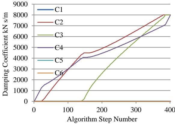
Figure 4 Evolution of damping coefficients with step (fixed base model)
