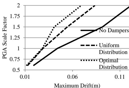
Figure 10 IDA for March 4<sup>th</sup> 1977 Earthquake, INCERC
