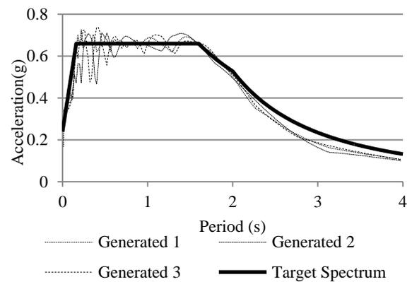
Figure 3 Generated accelerogram spectrum, target spectrum
