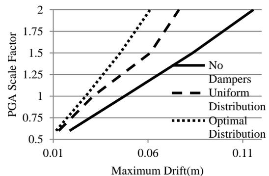
Figure 11 IDA for March 4<sup>th</sup> 1977 Earthquake, TUCB
