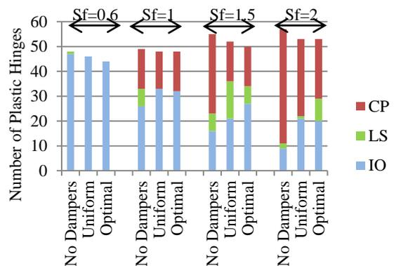
Figure 15 Number of Plastic Hinges for each  $S_f$  and distribution (INCERC)
