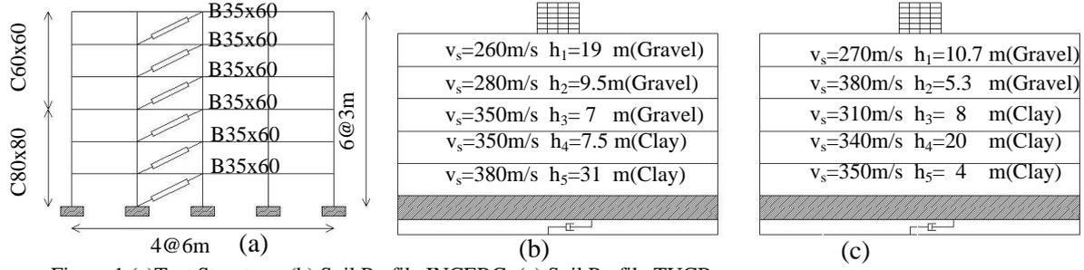
Figure 1 (a) Test Structure; (b) Soil Profile INCERC; (c) Soil Profile TUCB
