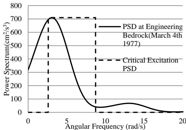
Figure 2 PSD of recorded motion, critical excitation
