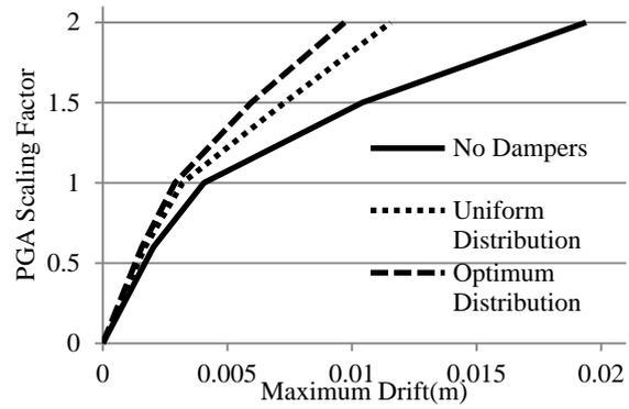
Figure 13 IDA for March 4<sup>th</sup> 1977 Earthquake, Fixed Base
