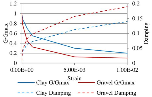
Figure 5 Evolution of G/Gmax and damping for considered soils
