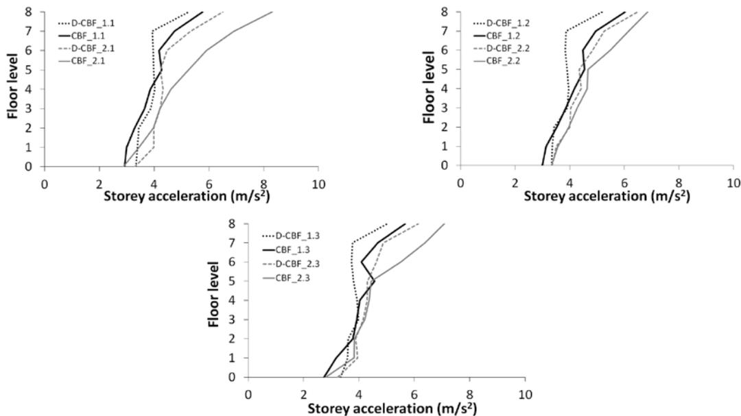
Figure 8. Storey acceleration pattern.
