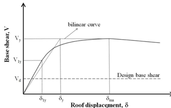
Figure 2. Capacity curves from pushover analysis
