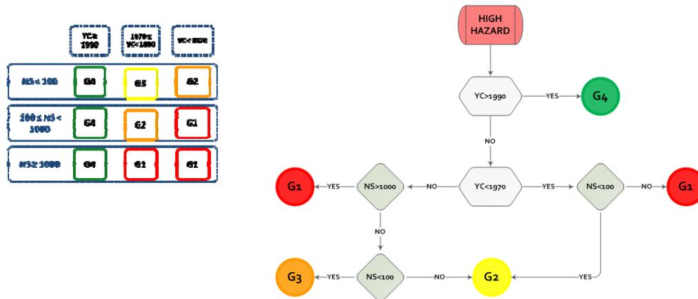
Figure 5.2. Schematic of Tier-1 screening procedure for high seismic hazard
