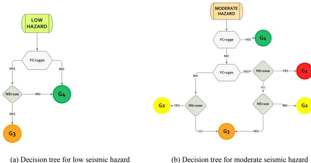
**Figure 5.1.** Schematic of Tier-1 screening procedure for low and moderate seismic hazard
