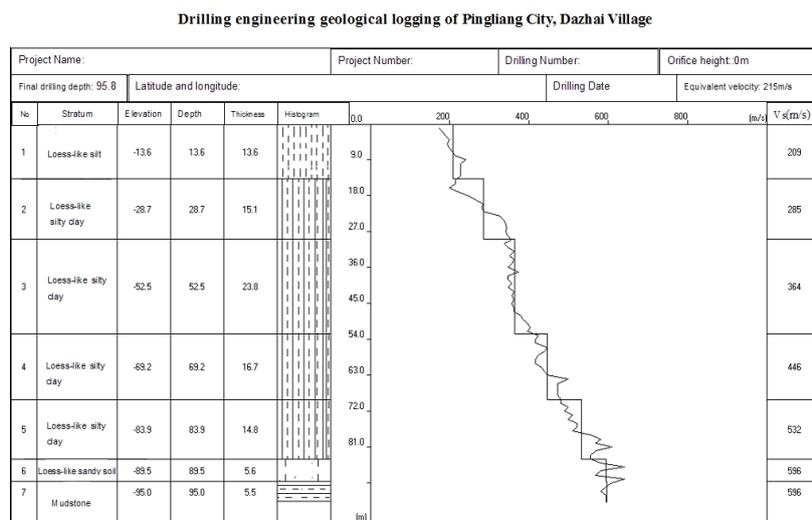
**Figure 8.** The borehole geologic records and Vs data of Pingliang city
