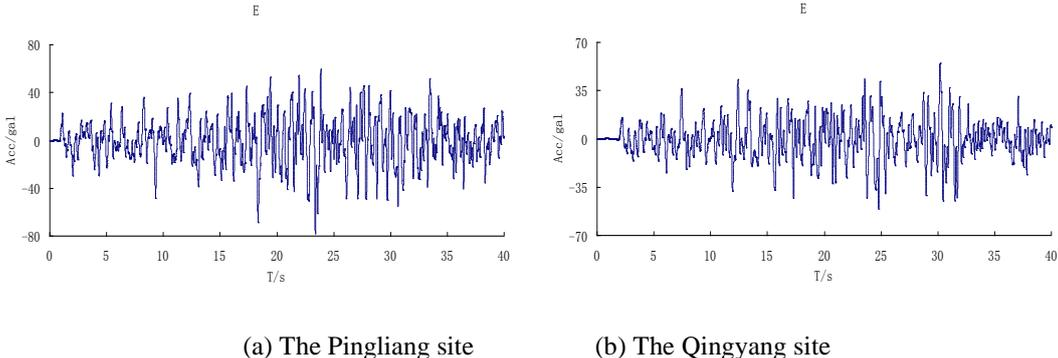
**Figure 15.** The acceleration-time curve of the point at the top of the loess Yuan
