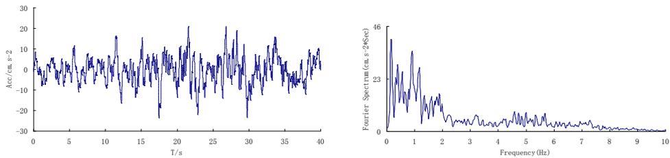
**Figure 12.** The far-field earthquake accelerogram and the FFT spectrum of the Wu Quanshan bedrock
