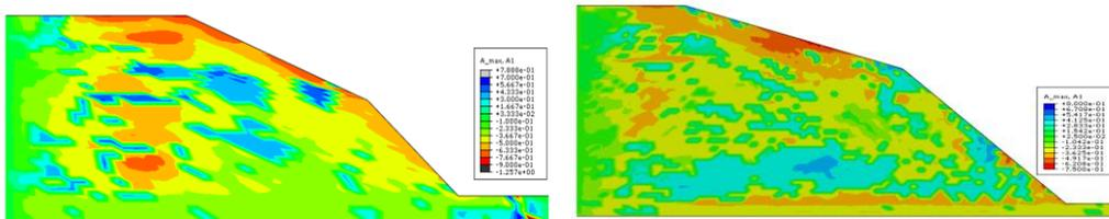
(a) The acceleration contours of Pingliang site (b) The acceleration contours of Qingyang site
