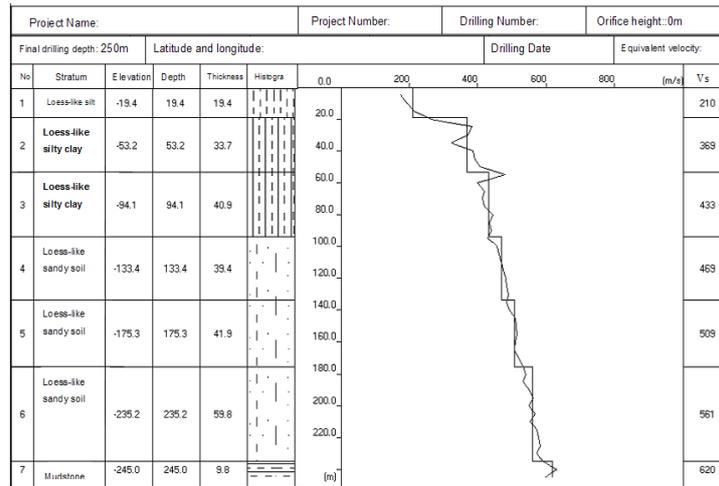
**Figure 9.** The borehole geologic records and Vs data of Qingyang city
