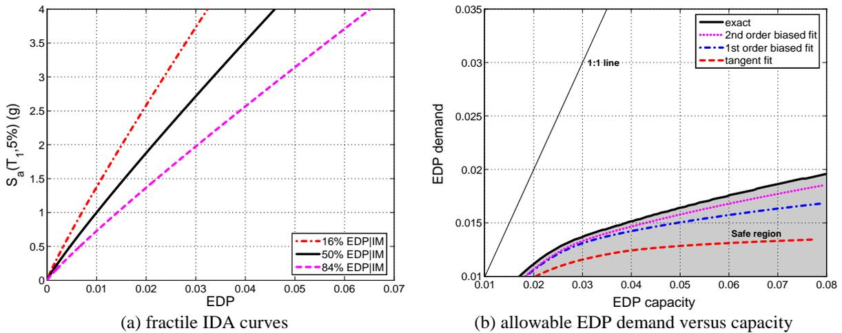
**Figure 5.3.** The DCFD comparison results for Building B, a high-curvature, ‘bad case’ ( $T_1 = 2.4s$ ,  $EDP = 0.01S_a^{1.1}$ , dispersions of 0.35 for demand and capacity)
