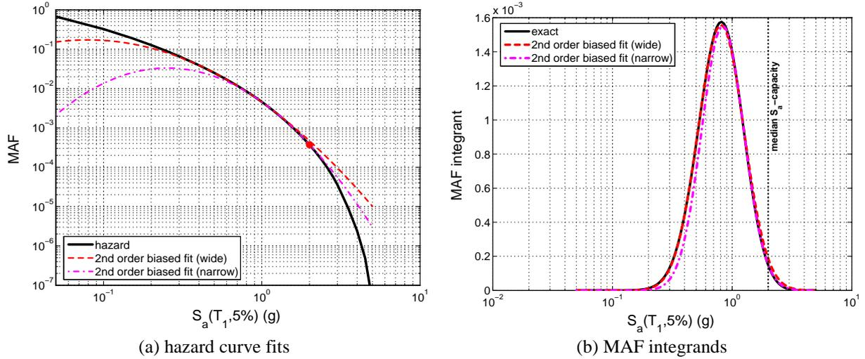
**Figure 4.1.** Two biased 2<sup>nd</sup> order power law fits, on a narrow or a wide interval, and the corresponding MAF integrands for a median  $S_a$ -capacity of 2g with 0.5 dispersion at the Van Nuys site ( $T_1 = 0.7$ s)
