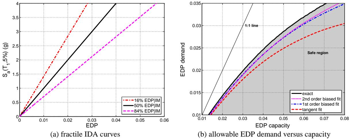
**Figure 5.2.** The DCFD comparison results for Building A, a low-curvature, ‘good case’ ( $T_1 = 0.7s$ ,  $EDP = 0.01S_a^{1.0}$ , dispersions of 0.35 for demand and capacity)
