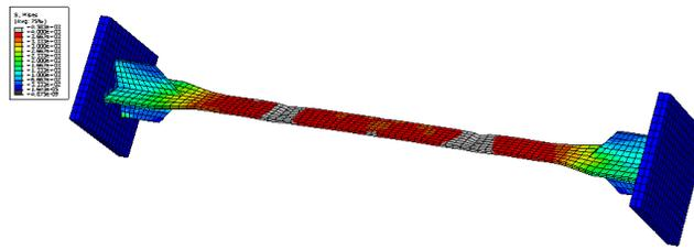
**Figure 15.** Deformed shape and Von Mises stress of RLBRB at maximum compressive displacement
