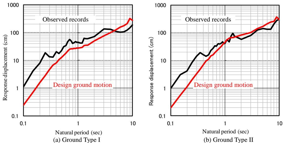
**Figure 2.2.** Displacement response of the observed acceleration records
