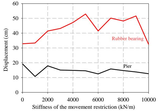
**Figure 3.4.** Displacement of the pier and the rubber bearing
