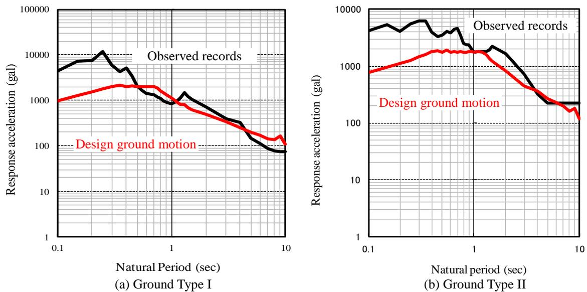
**Figure 2.1.** Acceleration response of the observed records
