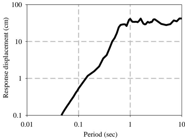
**Figure 3.3.** Response displacement of the input acceleration
