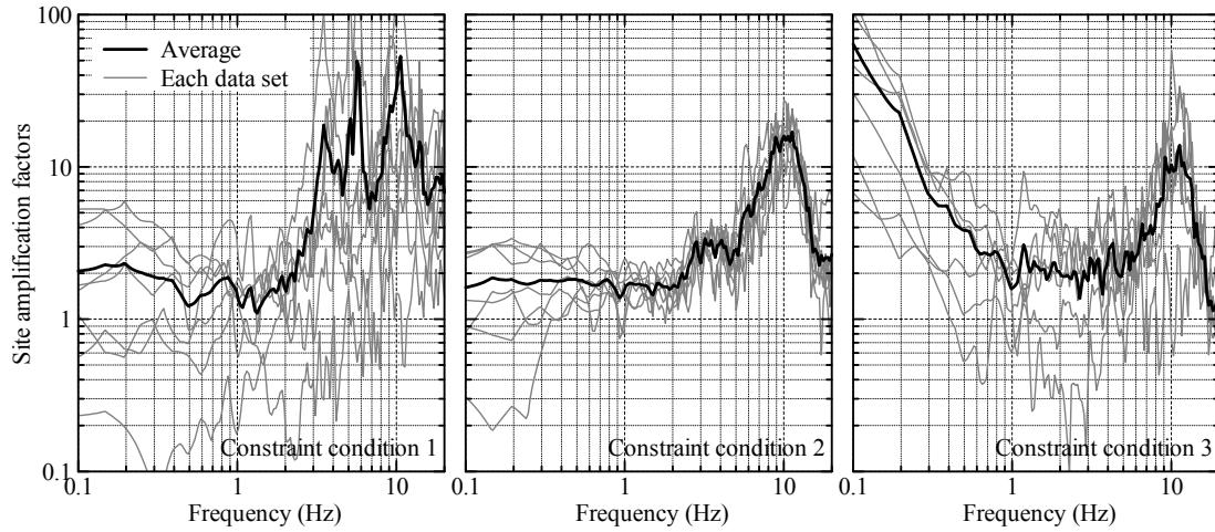
Figure 3.3. Difference in site amplification characteristics depending on the constraint condition.
