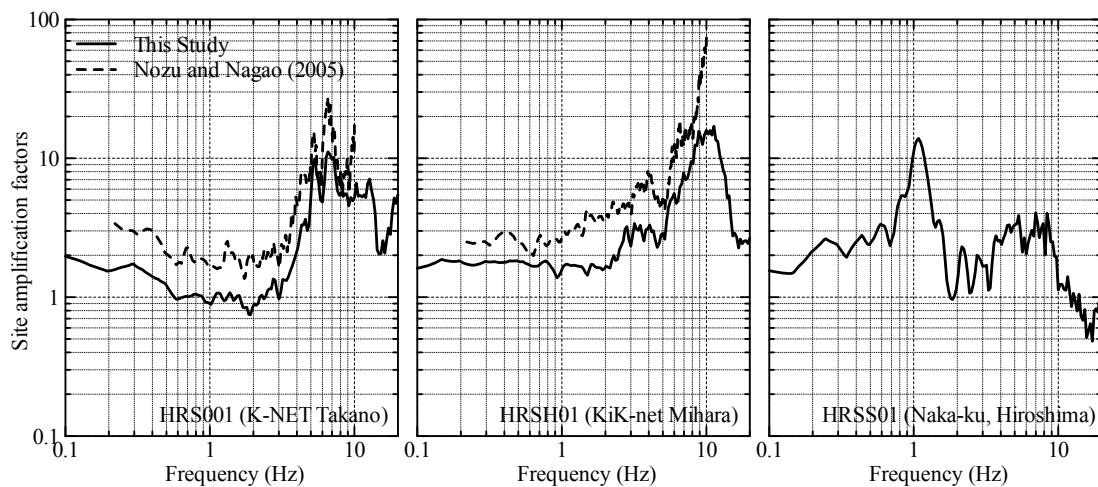
Figure 3.6. Comparison with the site amplification characteristics from Nozu and Nagao (2005).
