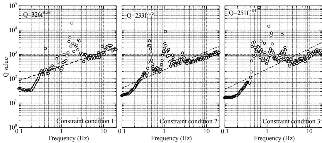
Figure 3.5. Difference in Q value depending on the constraint condition.
