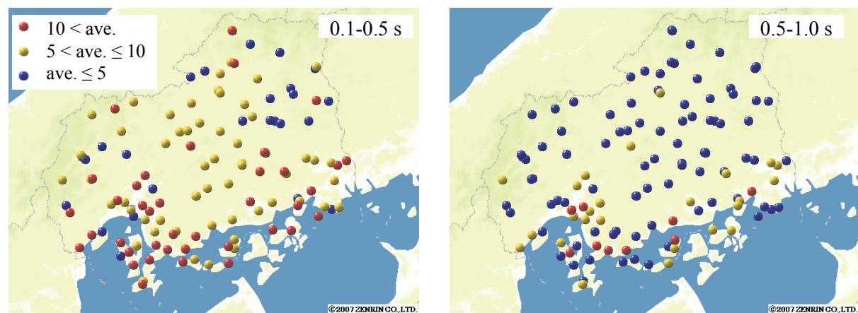
Figure 4.1. Distribution of average amplification factor for estimated site amplification characteristics.
