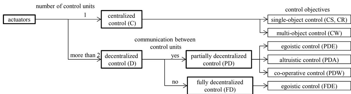
Figure 2.1. Basic concept of the classification of the control schemes for a building–equipment system
