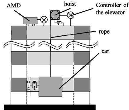
Figure 1.1. Model of the building–elevator system used in this study
