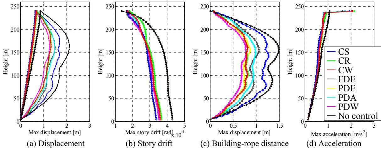
Figure 6.1. Maximum response of the mass points and nodes
