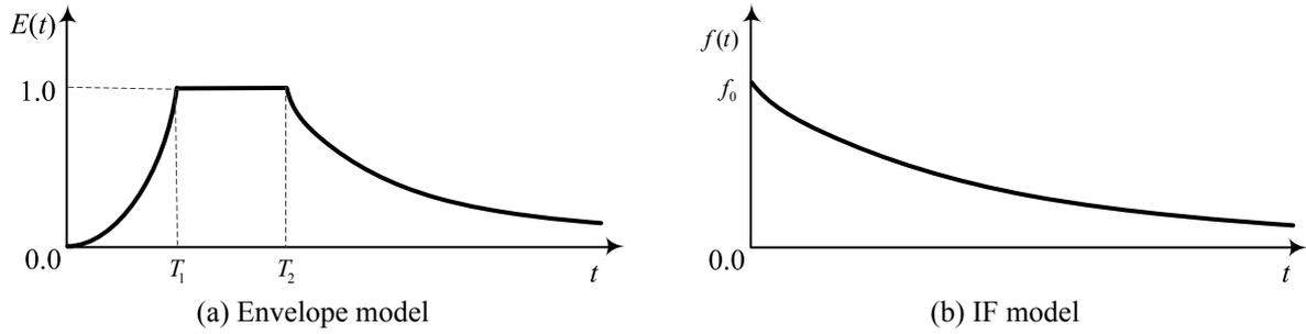
**Figure 2.1.** Envelope model and IF model of ground motions
