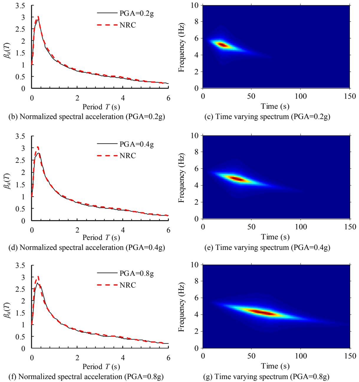
**Figure 4.5.** Time history, spectral acceleration and time varying spectrum of Type II ground motions
