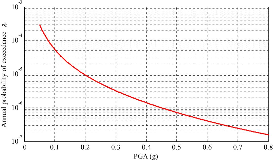
Figure 4.7. Seismic hazard curve
