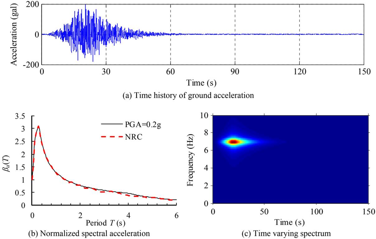
**Figure 4.4.** Time history, spectral acceleration and time varying spectrum of Type I ground motion
