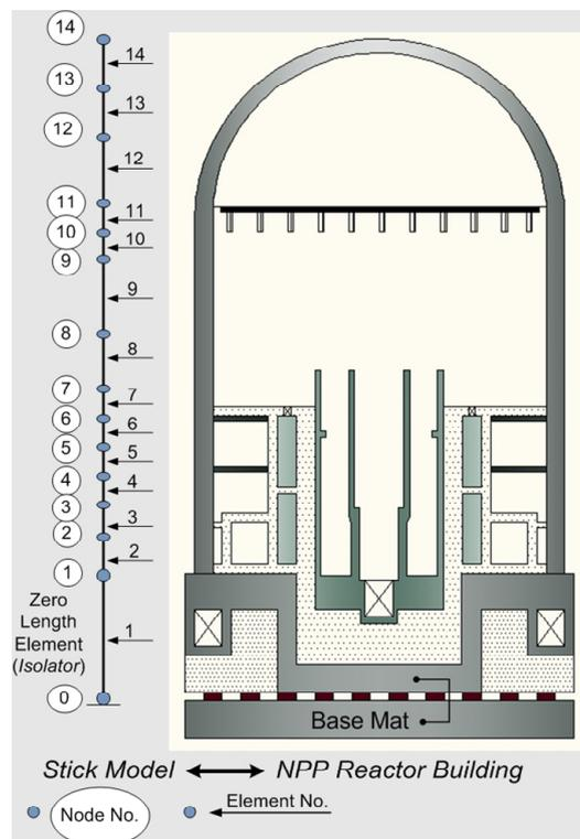
**Figure 4.1.** The section view of the base isolated NPP and its corresponding stick model
