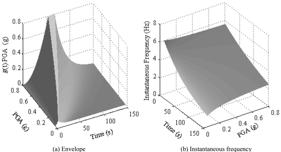
**Figure 4.3.** Change of envelope and instantaneous frequency with PGA
