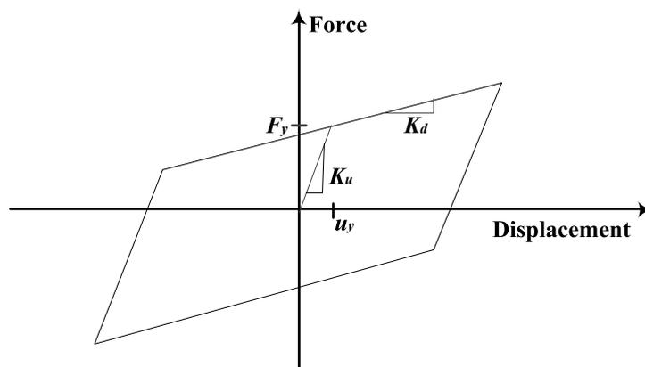
**Figure 4.2.** Bilinear hysteretic model of the base isolator
