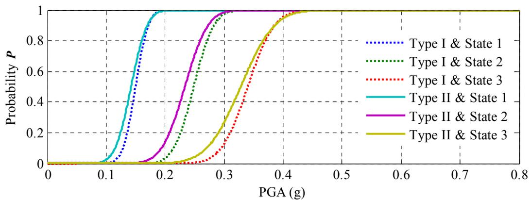
**Figure 4.6.** Fragility curves of the NPP under two types of ground motions
