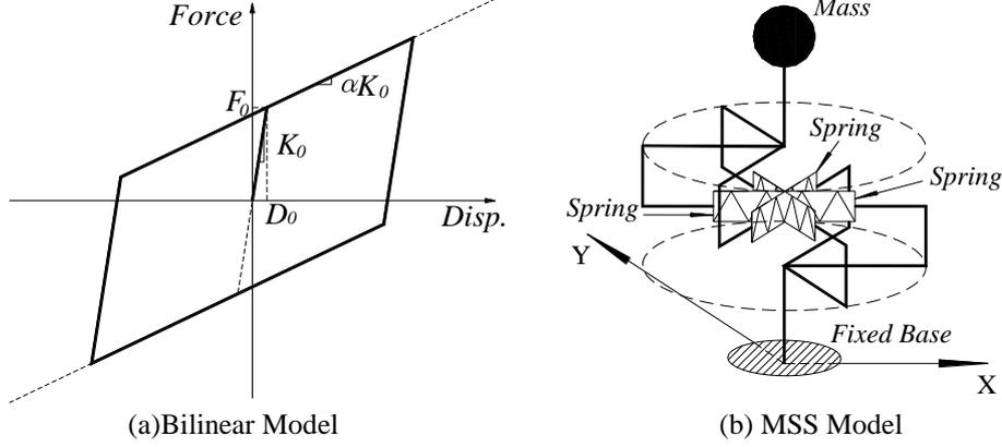
**Figure 7.** Hysteretic force-displacement relationship by hybrid simulations
