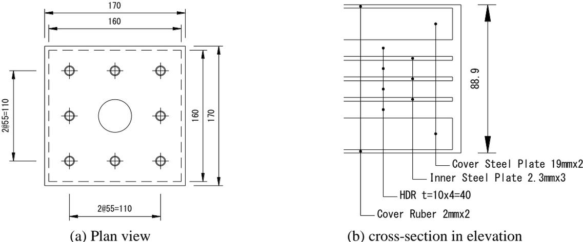
**Figure 1.** Plan view and cross-section in elevation of rubber bearing specimen
