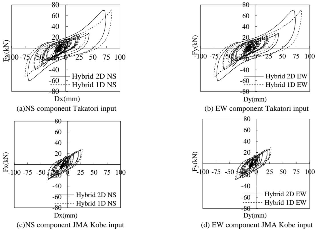
**Figure 6.** Hysteretic force-displacement relationship obtained by hybrid simulations
