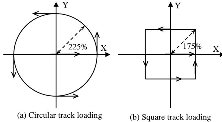
**Figure 3.** Bi-directional loading tracks
