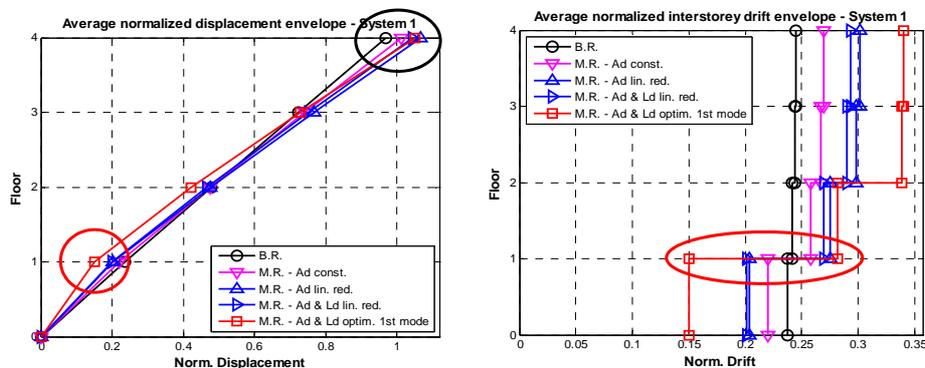
**Figure 6.1** Four-storey buildings: average value of the normalized displacement (left) and drift (right).
