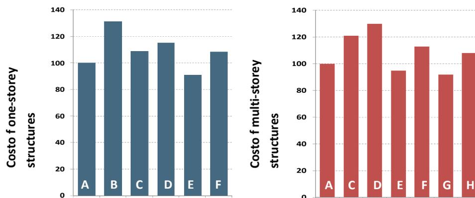
**Figure 7.1** Comparison of the costs of the examined structures: A = hinged frames, B = top isolation, C = friction devices, D = viscous-elastic dampers, E = partially fixed connections, F = D + E, G = perimeter walls, H = perimeter walls with controlled multi-rocking mechanism.
