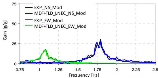
**Figure 4.5.** FRFs for 2DOF+TLD, correlation between signals 1%
