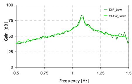
**Figure 2.10.** FRFs, low amplitude, deep TLD
