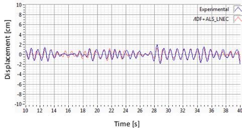
**Figure 4.1.** Displacement in x, 2DOF+TLD, correlation between signals 1% (Detail)
