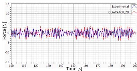
**Figure 2.7.** Dissipative force, high amplitude, shallow TLD (Detail)
