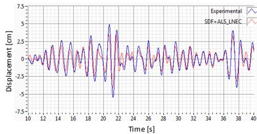
**Figure 3.3.** Displacements for SDF+ TLD, high amplitude (Detail)
