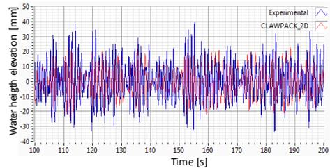
**Figure 2.3.** Water surface elevation, high amplitude, shallow TLD (Detail)
