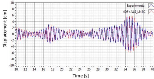
**Figure 4.3.** Displacement in y, 2DOF+TLD, correlation between signals 1% (Detail)
