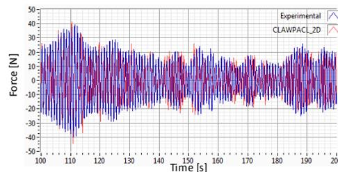
**Figure 2.8.** Dissipative force, high amplitude, deep TLD (Detail)
