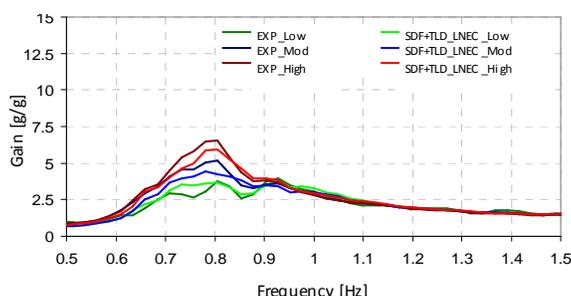
**Figure 3.5.** FRFs for SDF + TLD system (SDF approximate frequency of 0.81Hz)
