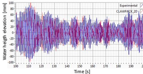
**Figure 2.4.** Water surface elevation, high amplitude, deep TLD (Detail)
