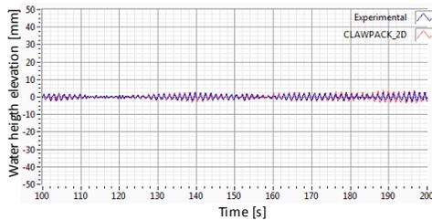
**Figure 2.1.** Water surface elevation, low amplitude, shallow TLD (Detail)
