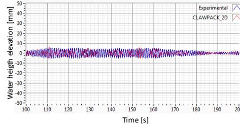
**Figure 2.2.** Water surface elevation, low amplitude, deep TLD (Detail)
