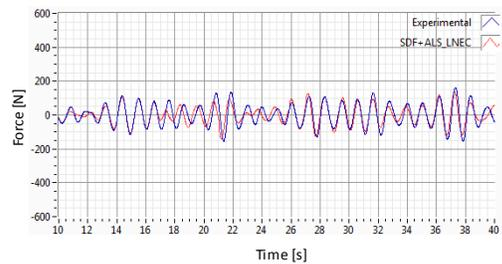
**Figure 3.2.** Dissipative forces for SDF+TLD, low amplitude (Detail)
