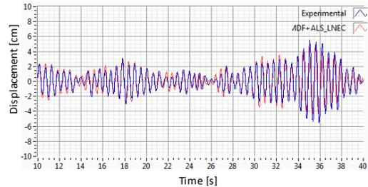
**Figure 4.4.** Displacement in y, 2DOF+TLD, correlation between signals 100% (Detail)
