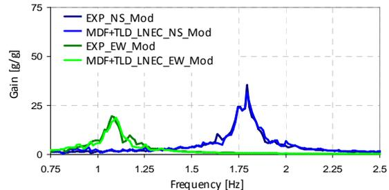
**Figure 4.6.** FRFs for 2DOF+TLD, correlation between signals 100%
