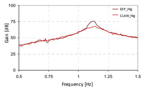
**Figure 2.12.** FRFs, high amplitude, deep TLD
