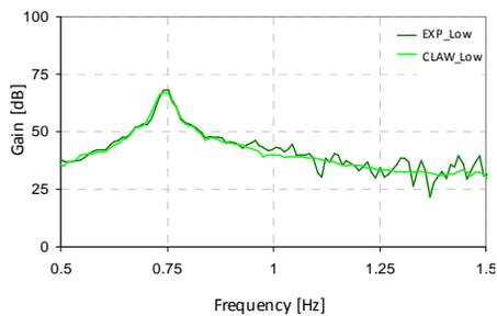
**Figure 2.9.** FRFs, low amplitude, shallow TLD
