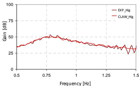
**Figure 2.11.** FRFs, high amplitude, shallow TLD
