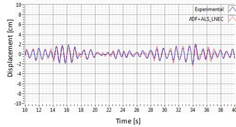
**Figure 4.2.** Displacement in x, 2DOF+TLD, correlation between signals 100% (Detail)
