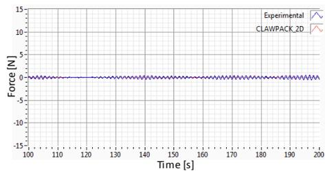
**Figure 2.5.** Dissipative force, low amplitude, shallow TLD (Detail)
