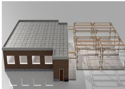
**Figure6:** Schematic overview on retrofitting by safe room pattern
