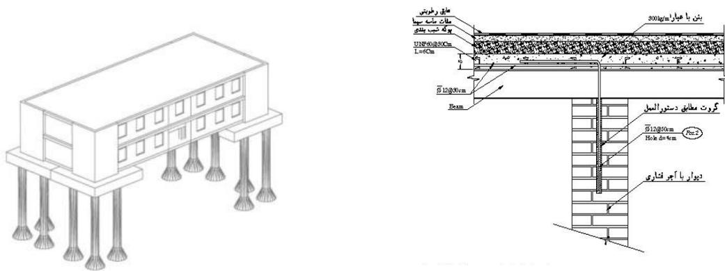
**Figure2:** Schematic overview and detail of retrofitting by shear wall pattern
