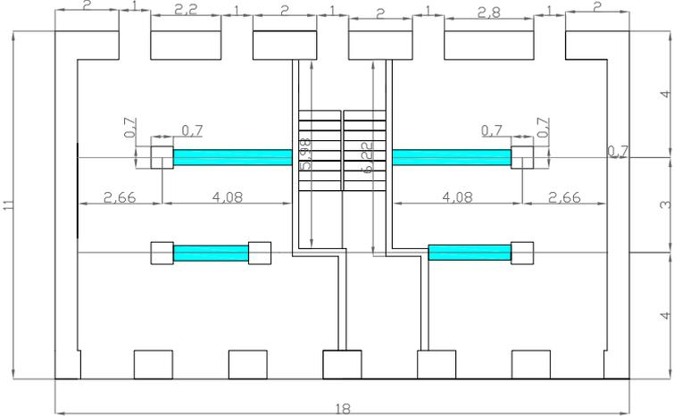
Figure 3.1. Positioning of the four shear walls on the ground floor – units in metres
