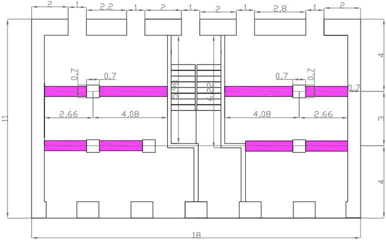
Figure 3.2. Positioning of the eight steel frames on the ground floor – units in metres
