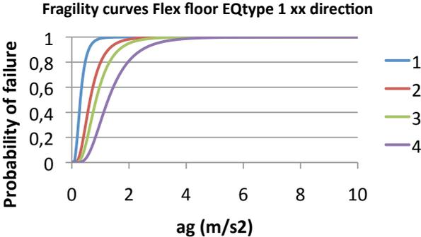
**Figure 6.1.** Fragility curve for earthquake type 1 in the xx direction for original building
