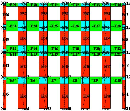
Figure 2.2. Equivalent frame idealization of front façade (P2)
