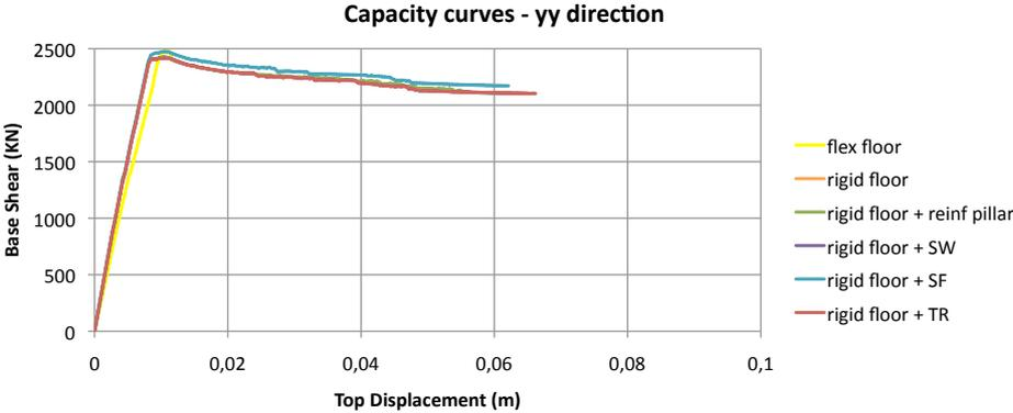
Figure 5.2. Pushover curves comparison in the yy direction
