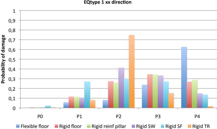
**Figure 6.2.** Probability of damage for earthquake type 1 in the xx direction
