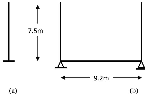
**Figure 11.** Analytical models of towers as (a) cantilever model, and (b) U frame model
