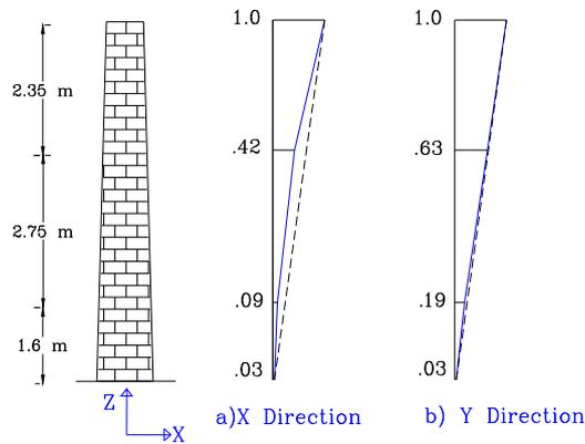
**Figure 10.** First vibration mode of left tower in a) X direction and b) Y direction
