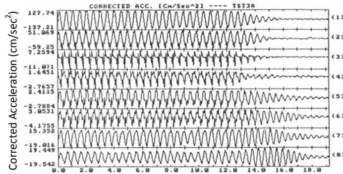
**Figure 6.** Forced vibration acceleration time histories recorded from Test 3A
