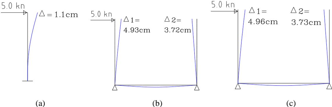
**Figure 13.** Lateral displacements of different models (a) cantilever, and (b) U frame without joint and (c) U frame with joint
