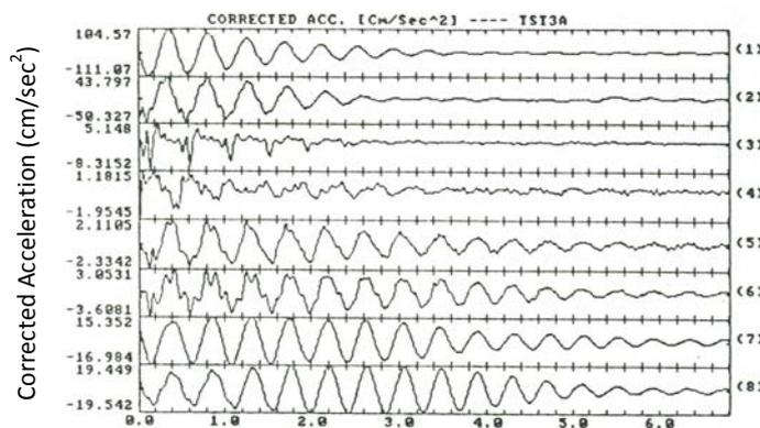
**Figure 8.** Free vibration acceleration time histories recorded from Test 3A
