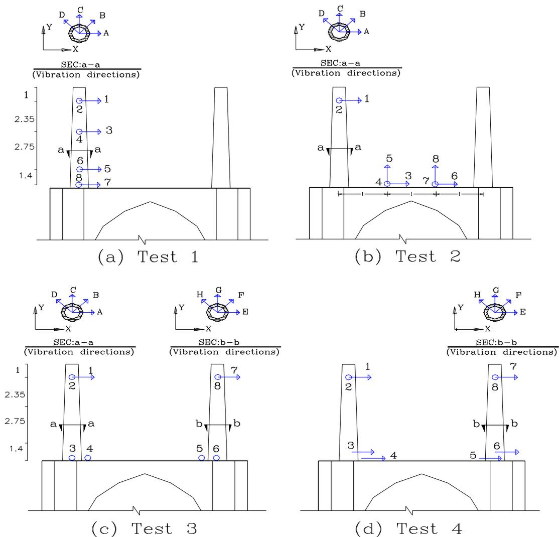
**Figure 5.** Arrangement of the accelerometers and vibration directions in different test series
