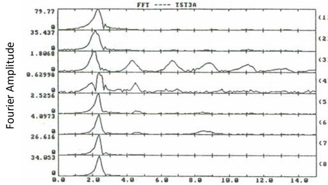
**Figure 9.** Free vibrations Fast Furrier Transformation (FFT) of Test 3A
