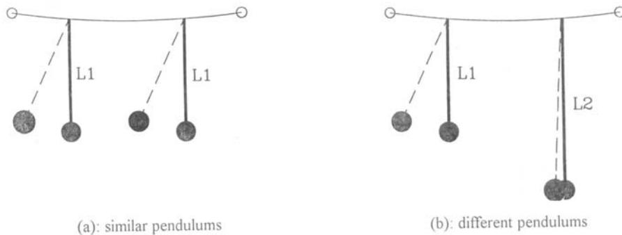
**Figure 4.** Resonance phenomena in vibration of similar pendulums
