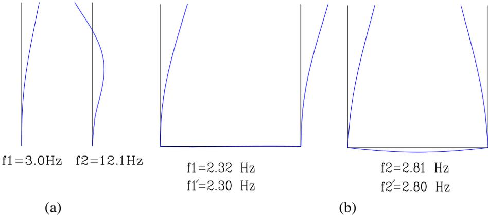
**Figure 12.** Frequencies of the first and the second modes of (a) cantilever models, and (b) U frame model with and without joint
