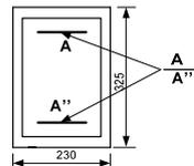
Note: width and depth of beams is 230 mm and 325 mm, respectively.
