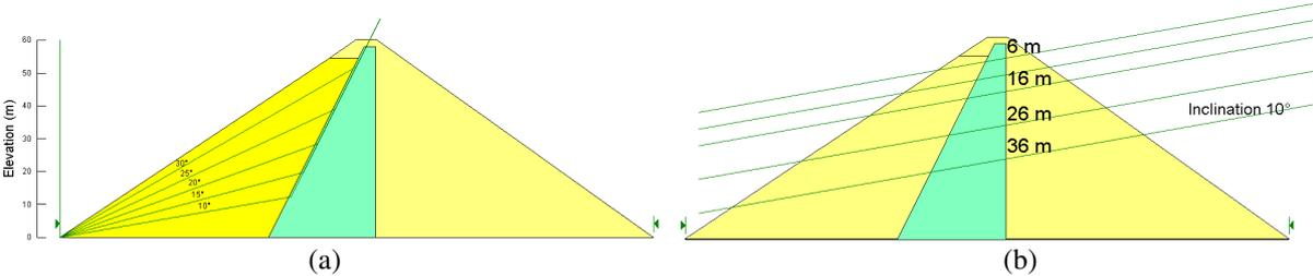
**Figure 5.3** Slip surfaces considered to estimate the stability of the dam slope and permanent deformation. (a) Slip surfaces with different inclination in the upstream shell. (b) Slip surfaces with 10° inclination through the dam. The distance from dam crest to the intersection with the boundary between the downstream shell material and the core is labelled .
