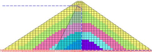
**Figure 5.1** 2D Finite element model of the dam. Zones with different material properties. G reduction functions and damping functions defined for an effective stress of 50 kPa, 100 kPa, 200 kPa, 300 kPa and 400 kPa.
