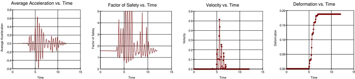
**Figure 5.2** Evaluation of the permanent deformation – an example. History plots of the stability factor, average acceleration (m/s<sup>2</sup>), velocity (m/s) and deformations (m) versus time (in seconds) for sliding surface with 30° inclination subjected to earthquake J1.
