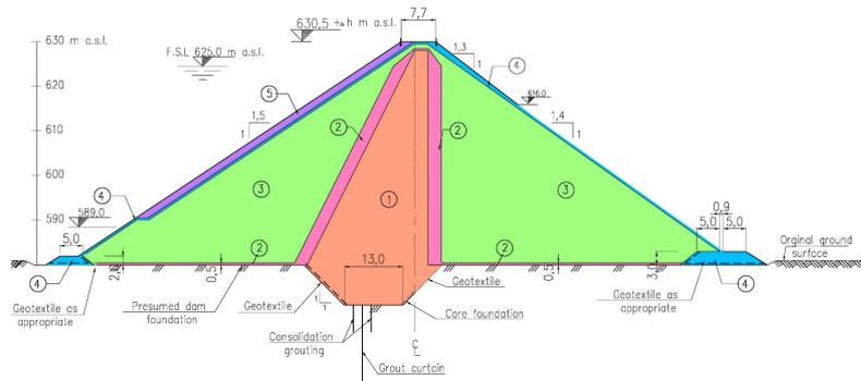
**Figure 3.1** A typical dam section showing the essential features. (1) Core; (2) Filter; (3) Shell; (4) Slope protection; (5) Riprap. The core trench shown is limited to the west abutment only.
