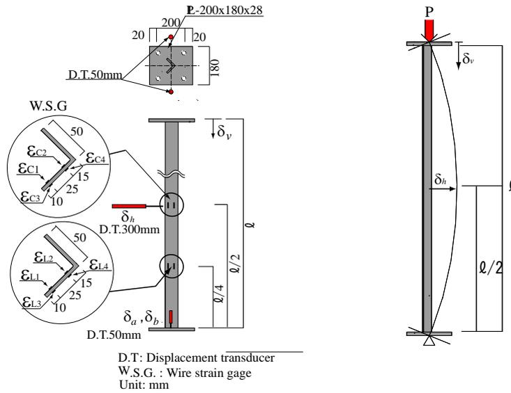
(a) Location of D.T. and W.S.G. (b) Schematic Illustration of measured values
