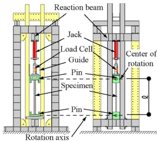
**Figure 2.** Concentrically axial loading test machine
