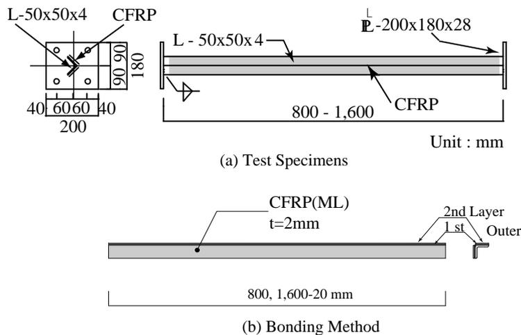
Figures 1(a),(b). Compression angle steel member bonding CFRP plates
