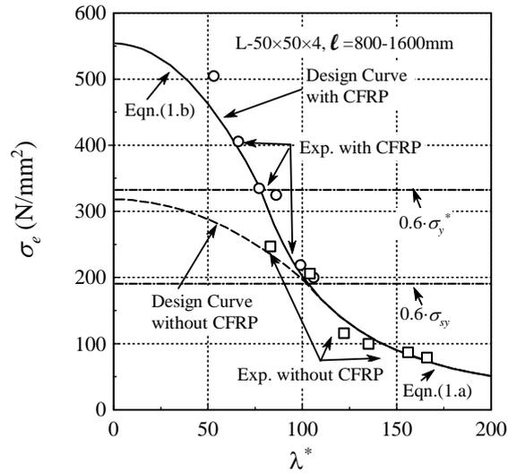
Figure 5. Comparison of compressive strength with formula and experiment
