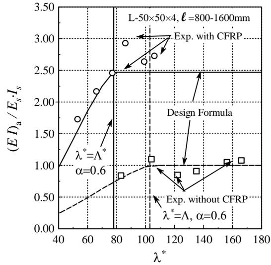
Figure 4. Relations between slenderness ratio and flexural rigidity from axial strength
