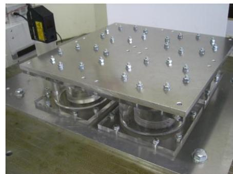
**Fig. 5.1.** Test Apparatus and Top View for Sliding Base Isolation Test by Shaking Table
