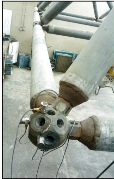
**Figure 3.3.** Three accelerometers to measure response of the grid in different directions
