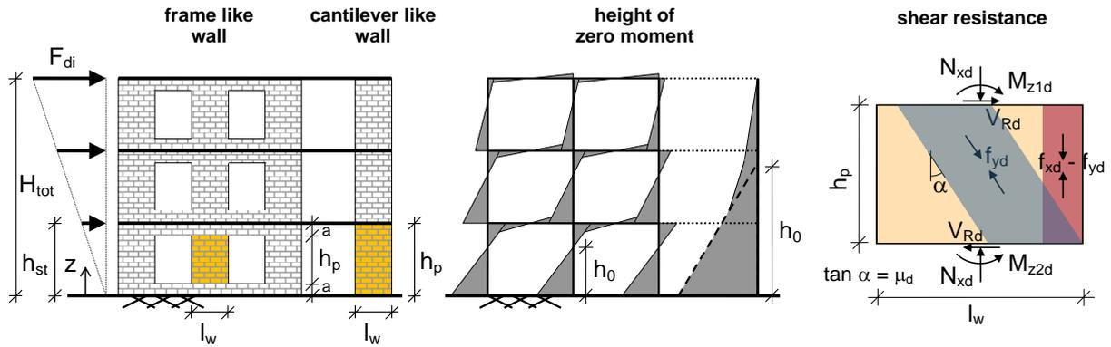
**Figure 3.1.** Nomenclature and definitions used for multi-storey walls and calculation of shear resistance  $V_{Rd}$
