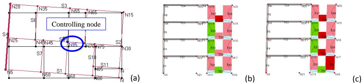
**Figure 4.3.** "3muri M3" in positive transverse direction: displacement figure (a), failure of first parapet between wall no. 1 and wall no. 2 (b) and failure of first vertical element; wall no. 1 (c)
