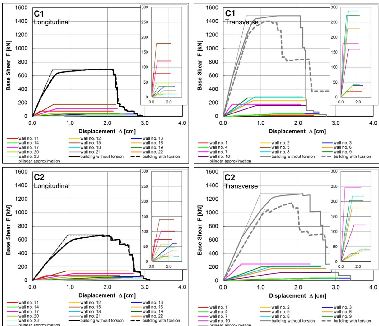
**Figure 3.3.** Pushover curves of the individual walls and the building using the calculation procedures C1 and C2
