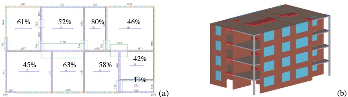
**Figure 4.1.** Load transfer in principal directions (longitudinal) of the slabs (a); overview of the 3muri model (b)
