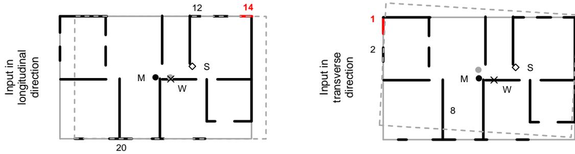
**Figure 3.4.** Displacement figure in ground view for the state of first wall failure (method SIA C2), Red: first wall failure and corresponding wall no., additionally stated wall no.: subsequent wall failures, M: centre of mass, W: centre of resistance, S: centre of stiffness
