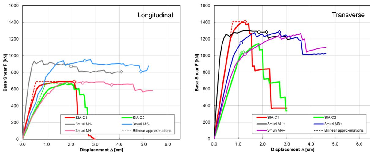
**Figure 5.1.** Comparison of pushover curves of three 3muri models and of the analytical calculations
