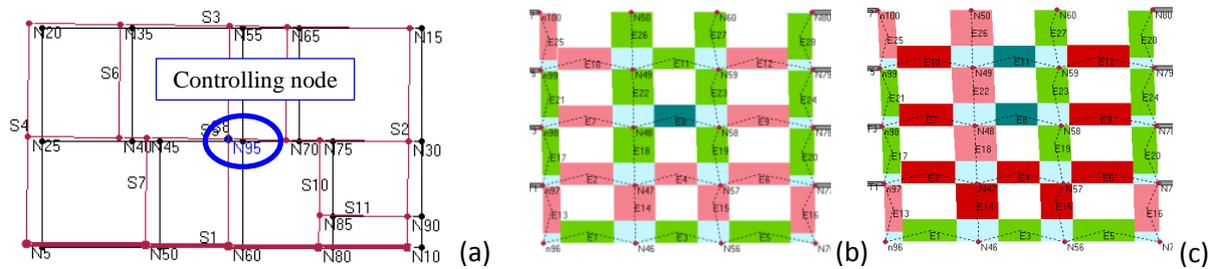
**Figure 4.2.** "3muri M3" in negative longitudinal direction: displacement figure (a), failure of first parapet between wall no. 20 and wall no. 21 (b) and failure of first vertical elements; wall no. 20 and wall no. 21 (c)
