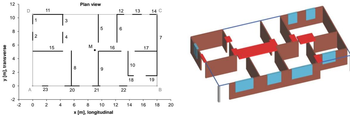
**Figure 2.1.** Idealized plan view of the building, numbering of the walls and corners; rendered view of one floor
