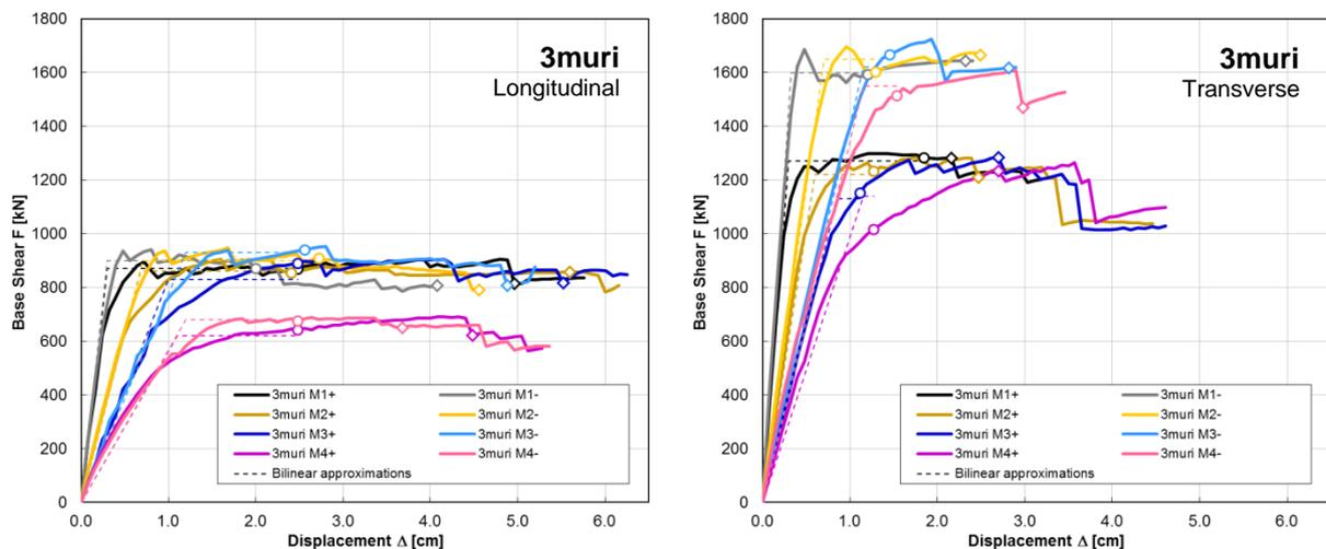
**Figure 4.4.** Pushover curves of the four 3muri models, for each input direction in positive and negative direction. The circle marks first parapet failure and the square first vertical wall failure.
