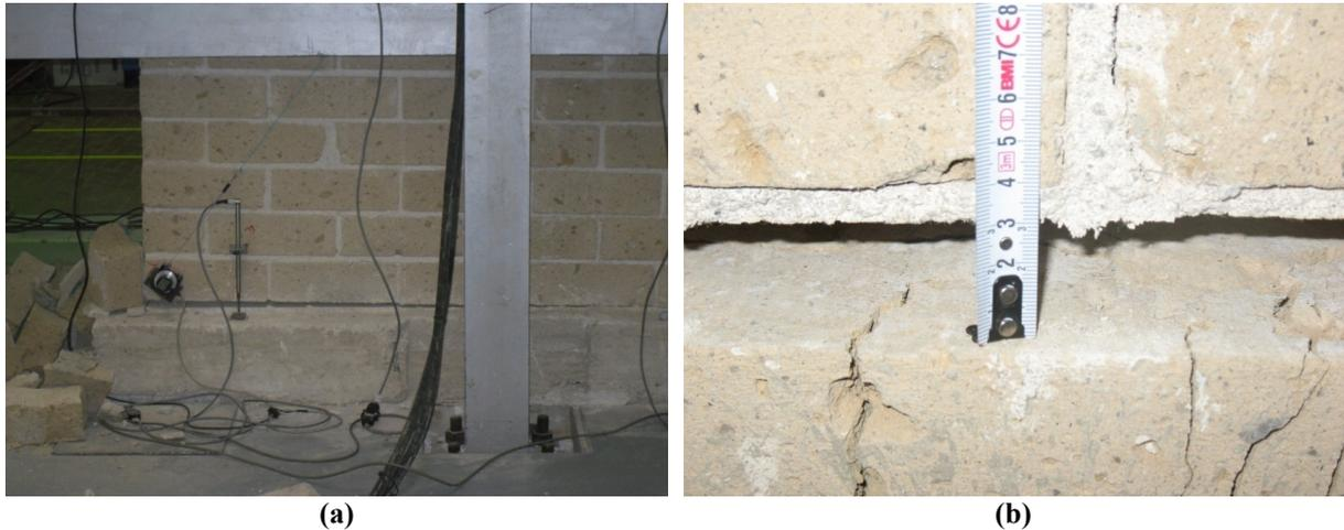
**Figure 8.** Rocking induced crack at pier base of specimen #2 ( $\theta = 2.24\%$ ): (a) front view; (b) crack width
