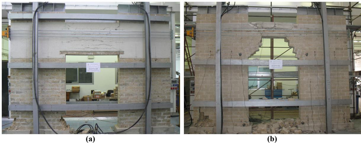
**Figure 9.** Overall damage at maximum lateral drift: (a) IMG-repaired specimen #1; (b) specimen #2
